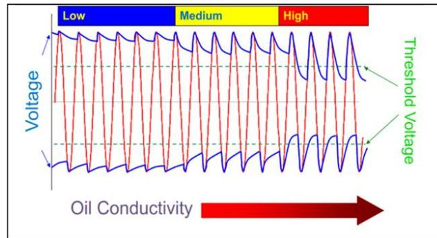
Figure 1. Voltage decay as a function of increased crude oil conductivity [9]
