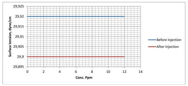
Figure 1. Demulsification Simulation #1: Effect on surface tension
