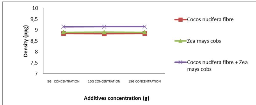
Fig. 3. Density of the various mud samples at different concentration
