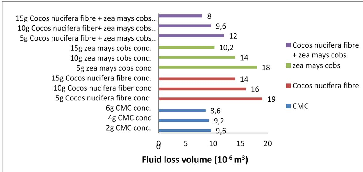
Fig. 4. Fluid loss volume of the various mud samples at different concentrations
