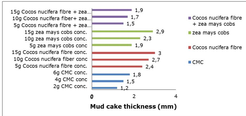
Fig. 5. Filter cake thickness for the various mud samples at different concentration
