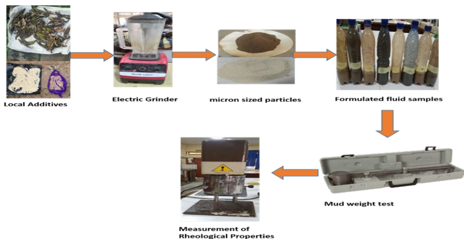
Figure 1. Experimental steps of drilling fluid preparation.
