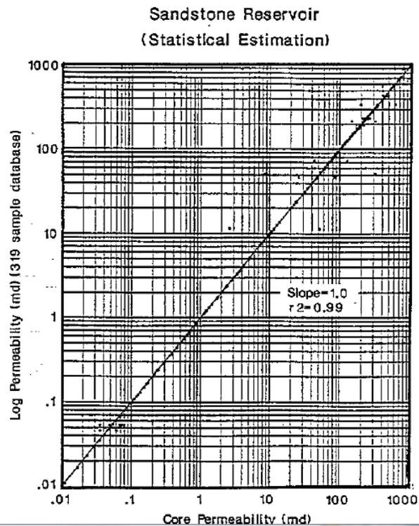
Figure 4 log vs. core permeability
