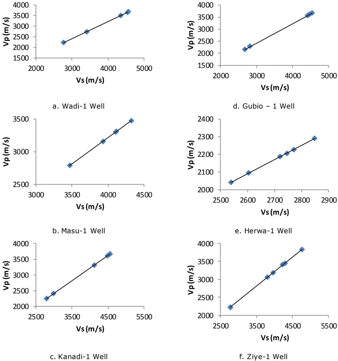
Fig. 3. Linear relationship between shear and compressional velocities
