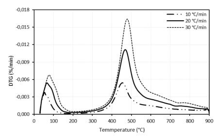
Figure 3. DTG (%) Mass loss plots for carbonisation of DDG coal
