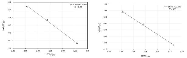
Figure 4. Kissinger kinetic plots for Drying DDG Coal
