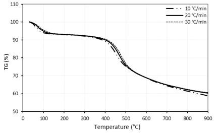
Figure 2. TG (%) Mass loss plots for carbonisation of DDG coal
