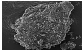
Figure 1. SEM Micrograph of Duduguru (DDG) coal
