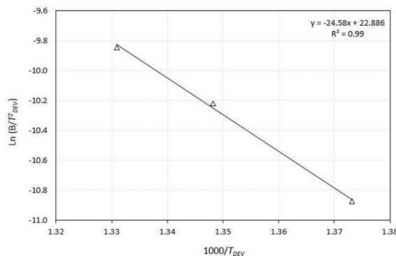
Figure 5. Kissinger kinetic plots for Devolatilization of DDG Coal
