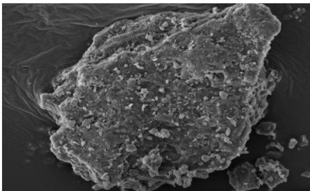
Figure 1. SEM Micrograph of Duduguru (DDG) coal
