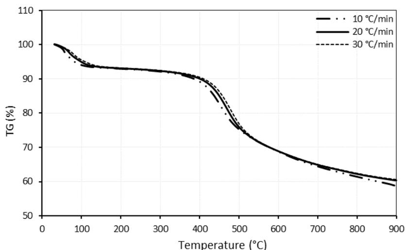
Figure 2. TG (%) Mass loss plots for carbonisation of DDG coal
