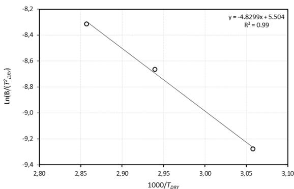
Figure 4. Kissinger kinetic plots for Drying DDG Coal
