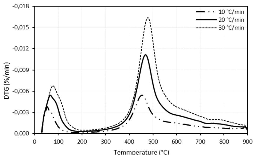
Figure 3. DTG (%) Mass loss plots for carbonisation of DDG coal
