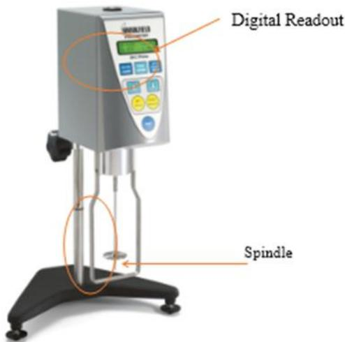
Figure 4. Brookfield DV-I™ prime viscometer
