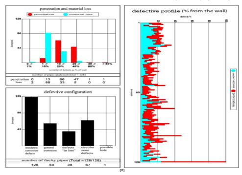
Figure 2. Damage regarding pipe body region penetration
