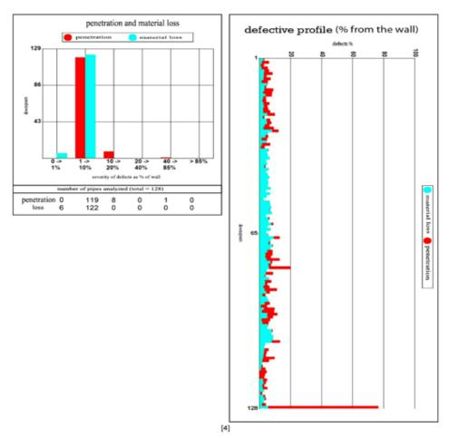
Figure 4. Damage regarding pipe joint projections
