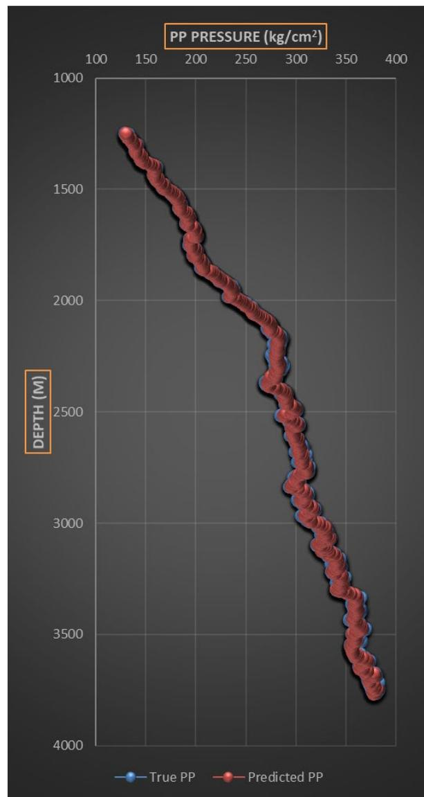
Figure 12. PP predicted vs. PP true for the developed model.
