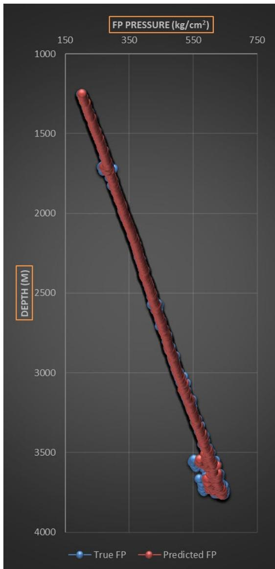
Figure 11. FP predicted vs. FP true for the developed model.
