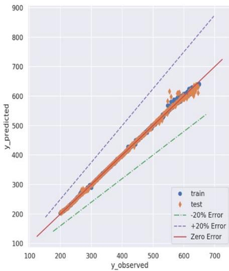
Figure 9. Regression plot of the true FP and predicted FP for train/test dataset for Ensemble model.
