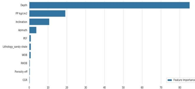
Figure 13. Features contribution to the fracture pressure prediction
