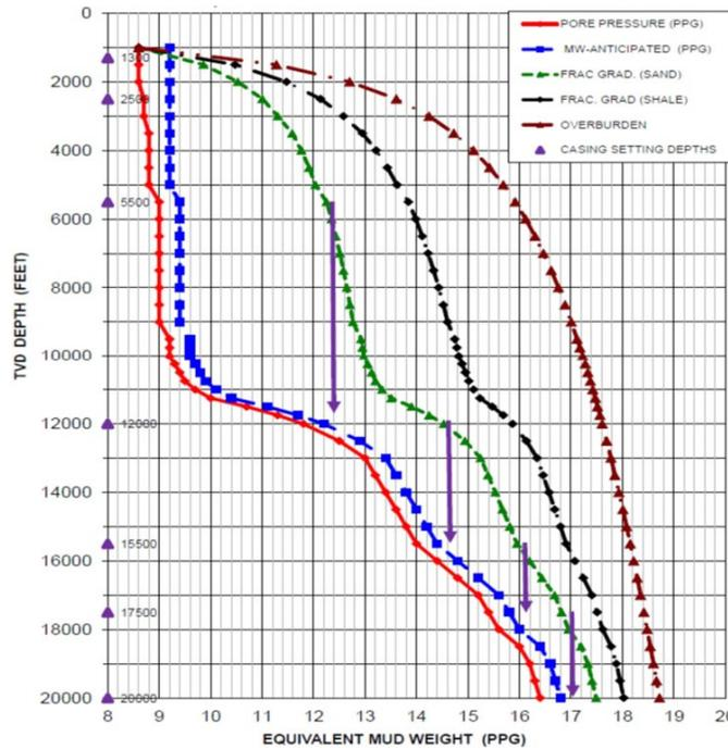
Figure 1. Depth (TVD) versus pore pressure gradient, anticipated mud weight, overburden pressure gradient, fracture gradient (shale & sand) and casing shoes.
