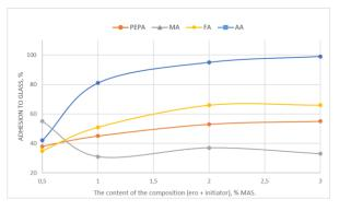
Figure 3. The dependence of the adhesion of the modified bitumen on the content of the composition [EPO: initiator]
