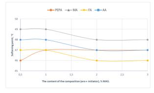
Figure 2. Dependence of softening temperature of modified bitumen on the content of the composition [EPO: initiator]
