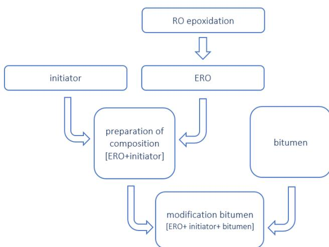
Figure 1. Scheme of bitumen modification by green epoxy rape oil
