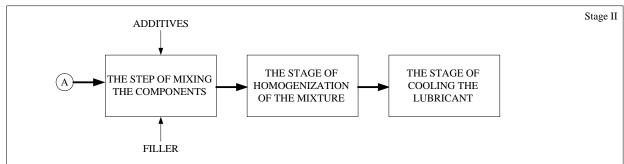
Fig. 4. The scheme for the grease production from secondary polyethylene raw materials
