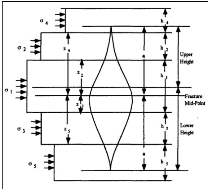
2D model to evaluate the fracture half-length and dimensionless fracture conductivity. Rahim considers asymmetric layers where the stress difference between upper and lower layers is equal with a given value of net pressure and reasonable values of zones thickness, fracture toughness Fig. 2.
