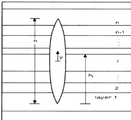
Fig. 1. Definition of variables for fracture containment problem [6]
