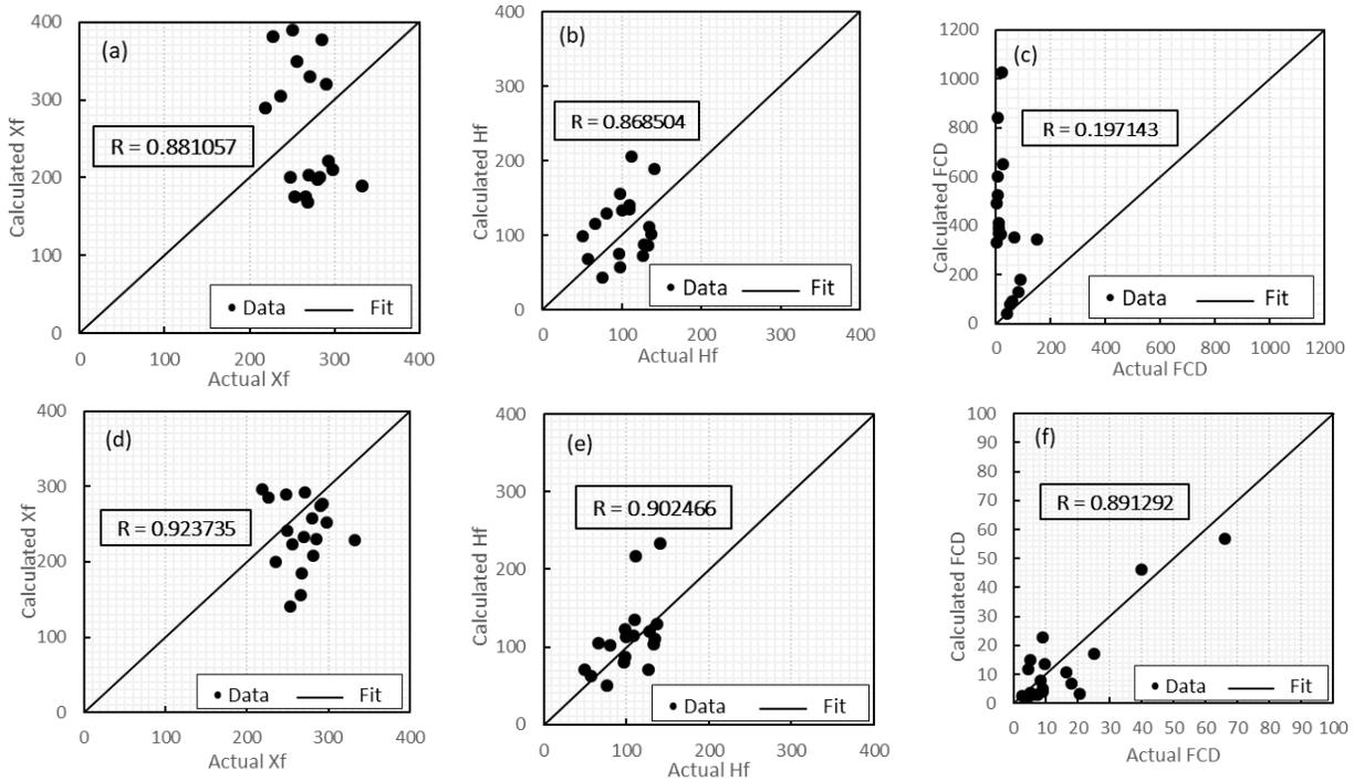
Fig. 5. ANN and Software comparison for fracture height, fracture half-length and fracture conductivity. (a) Software fracture half-length; (b) Software fracture height; (c) Software fracture conductivity; (d) ANN fracture half-length; (e) ANN fracture height; (f) ANN fracture conductivity
