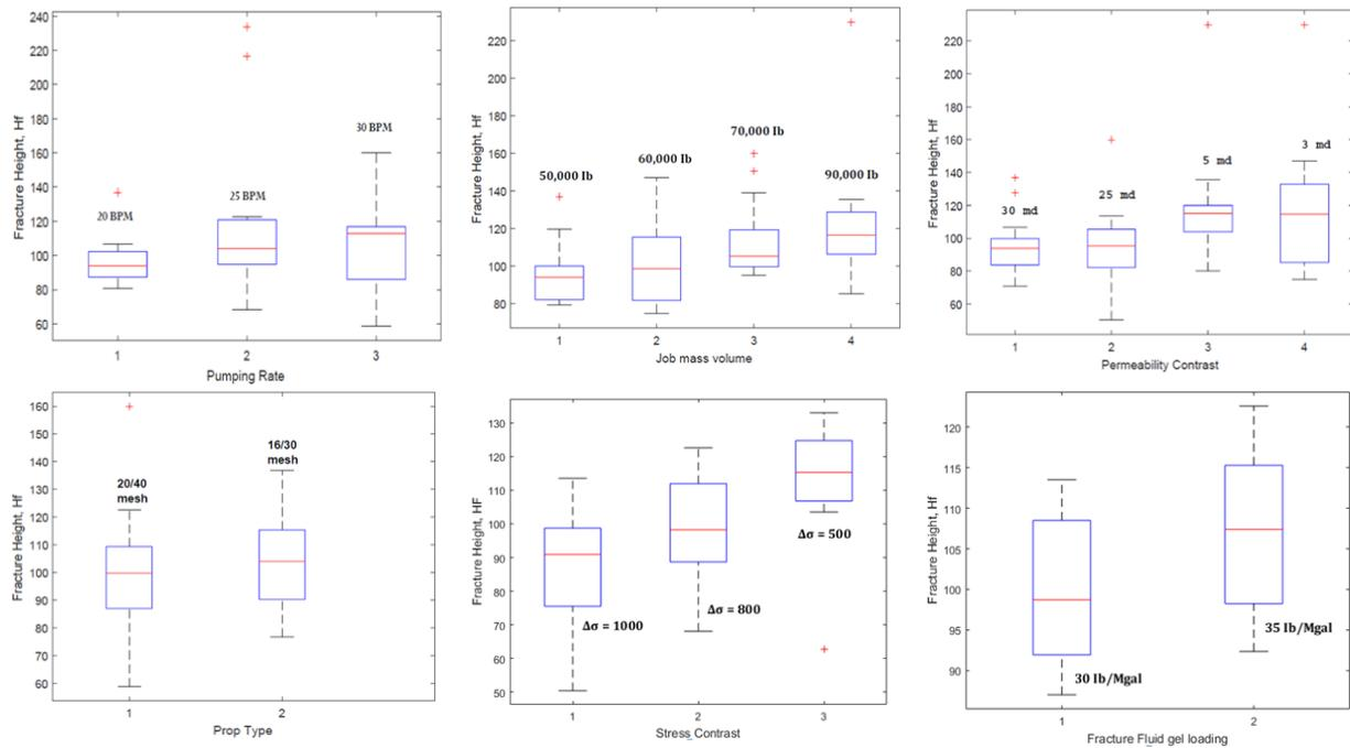
Fig. 7. Boxplots of effects of fracture stimulation parameters and rock properties on fracture height growth. (a) Pumping Rate; (b) Job mass volume; (c) Permeability contrast; (d) artificial barrier prop type; (e) stress contrast; (f) Fracture fluid gel loading (Generated by MATLAB™)
