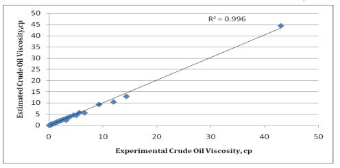
Figure A2: Cross plot for oil viscosity above bubble point ( $\mu_o$ , **BEALS**).
