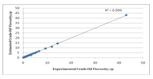
Figure A1: Cross plot for oil viscosity above bubble point ( $\mu_{oann}$ , **FFBPNN**).
