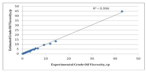
Figure A6: Cross plot for oil viscosity above bubble point (µ<sub>o</sub>, KARTOATMODJO-SCHMIDT)
