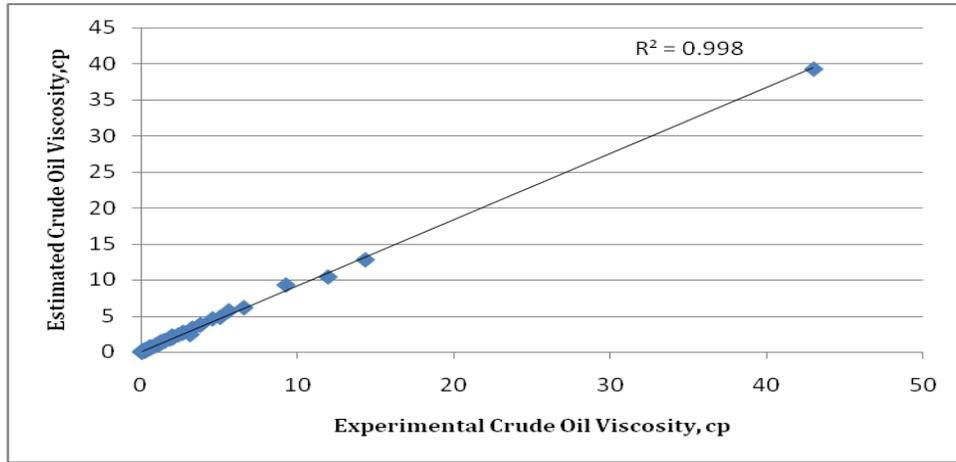
Figure A3: Cross plot for oil viscosity above bubble point ( $\mu_o$ , **KAHN**).
