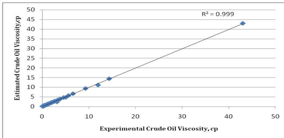
Figure A1: Cross plot for oil viscosity above bubble point ( $\mu_{oann}$ , FFBPNN).
