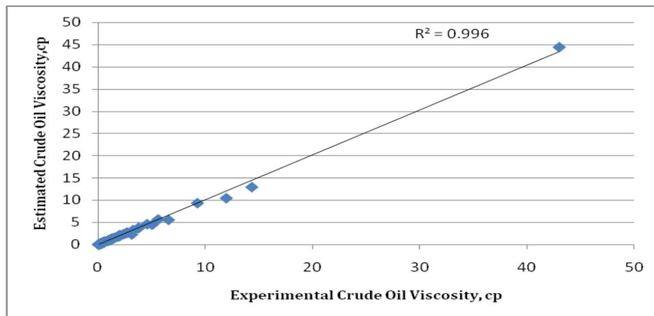
Figure A2: Cross plot for oil viscosity above bubble point ( $\mu_o$ , BEALS).
