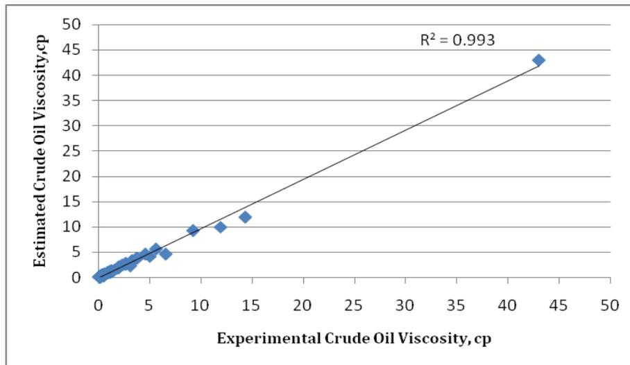
Figure A7: Cross plot for oil viscosity above bubble point ( $\mu_o$ , **R. ABEDINI**)
