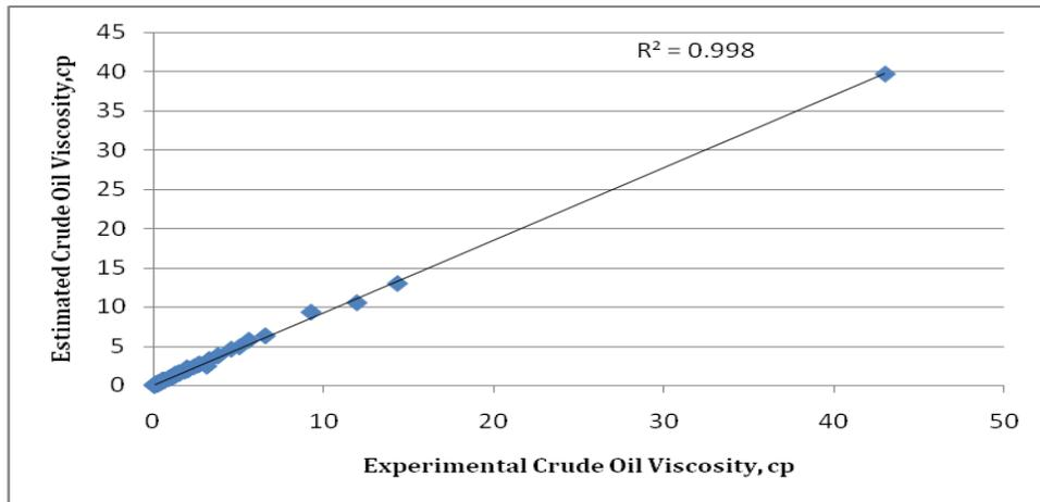
Figure A4: Cross plot for oil viscosity above bubble point ( $\mu_o$ , **ISEHUNWA**).
