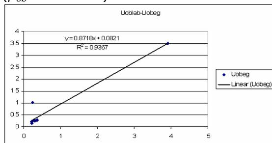
Fig. 5 Comparison of the estimated crude oil viscosity versus experimental crude oil viscosity (Begg-Robinson correlation).
