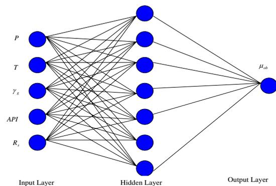
Fig. 2 A schematic of the achieved artificial neural network topology used for  $\mu_{ob}$
