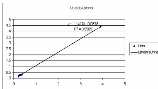
Fig. 3 Comparison of the estimated crude oil viscosity versus experimental crude oil viscosity ( $\mu_{ob}$  ANN model).
