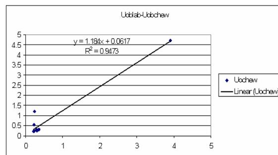
Fig. 4 Comparison of the estimated crude oil viscosity versus experimental crude oil viscosity (Chew-Connally correlation).
