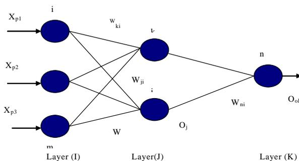
Fig. 1 One output layer back propagation neural network
