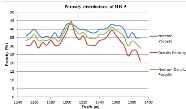
Figure 6. Porosity of HB-9 by various methods
