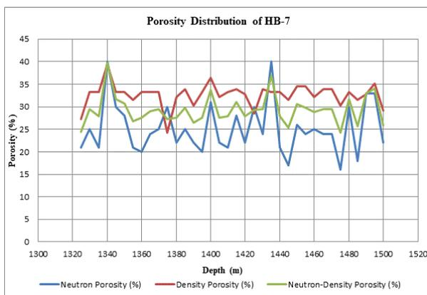
Figure 2. Porosity of HB-7 by various methods
