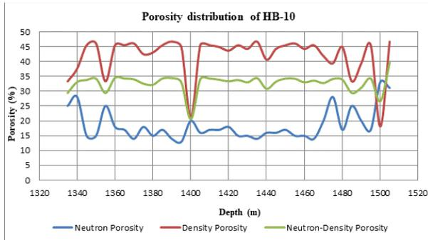
Figure 4. Porosity of HB-10 by various methods
