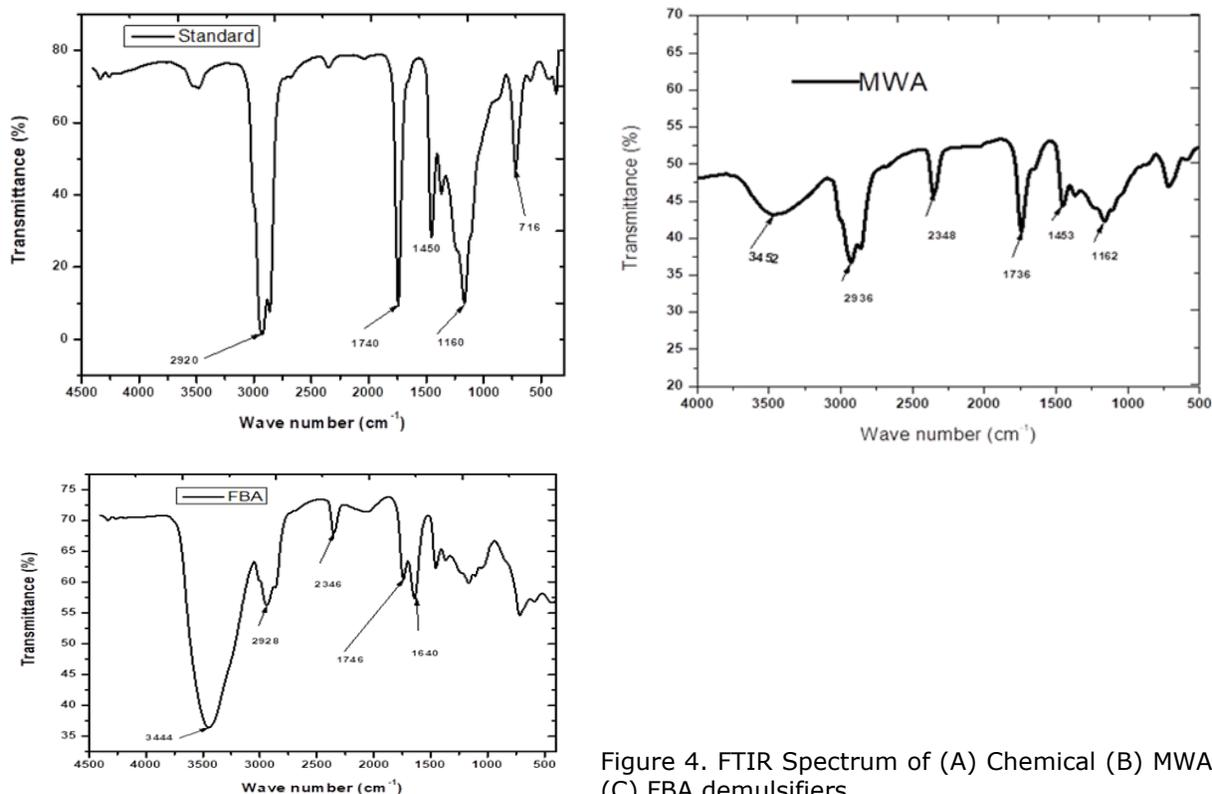
Figure 4. FTIR Spectrum of (A) Chemical (B) MWA (C) FBA demulsifiers.
