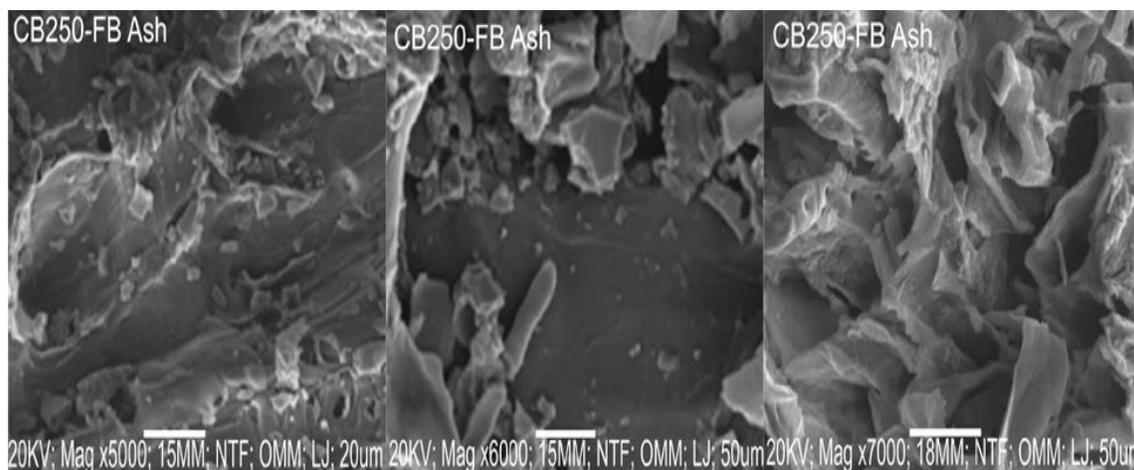
Figure 6. SEM analysis of furnace burn ash.
