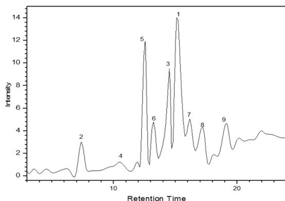
Figure 1. GC-MS spectrum of microwave ash (MWA) demulsifier.
