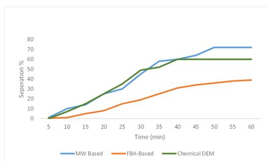
Fig. 8. Time and separation efficiency of the demulsifier.
