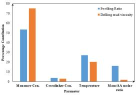
Figure 3. Percentage contribution of effective factors of swelling ratio and drilling mud viscosity
