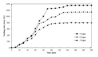
Figure 4. Equilibrium water uptake behavior of optimized hydrogel with various monomer content vs. time
