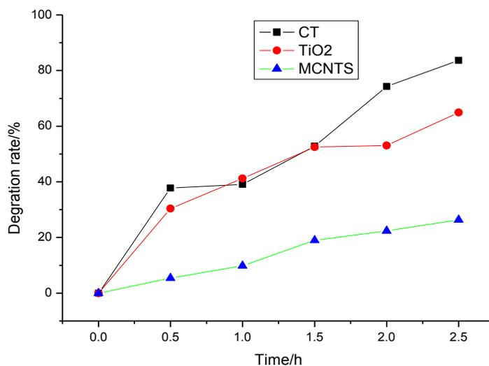
Fig 1. The photodegradation rate of MCNTs, TiO<sub>2</sub>, MCNTs-TiO<sub>2</sub> with an amount of 100mg of the methyl orange degradation
