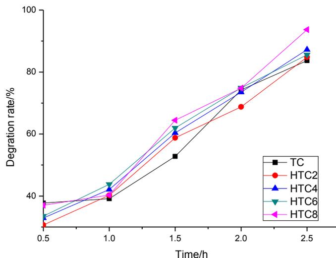
Fig 2. The photodegradation rate of various MCNTs-HPW//TiO<sub>2</sub> ratios with an amount of 100mg of the methyl orange degradation.
