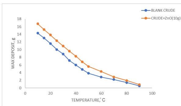
Figure 7. Cumulative wax deposit against temperature.
