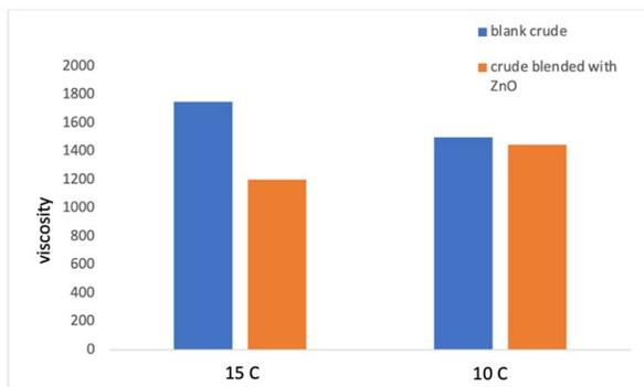
Figure 6. Viscosity of blank crude and viscosity of crude oil blended with zinc oxide against temperature (10 and 15°C).
