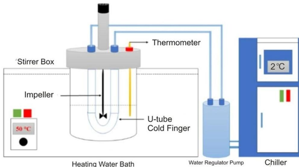
Figure 2. Schematic diagram of the cold finger apparatus.
