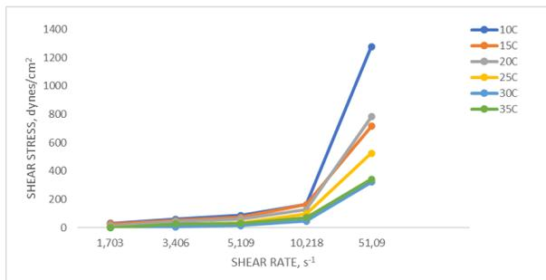
Figure 4. Plot of shear stress against shear rate of blank crude.
