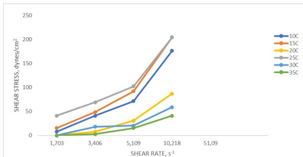
Figure 5: Plot of shear stress against shear rate of crude mixed with 10g zinc oxide.
