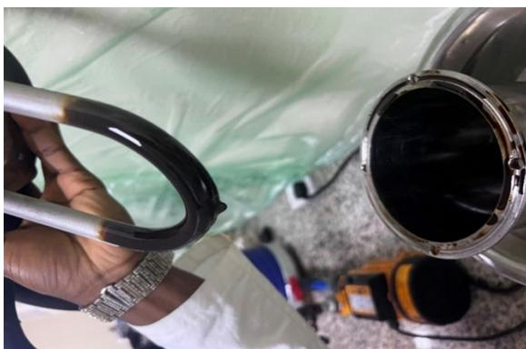
Figure 3. Wax deposit on U-tube.
