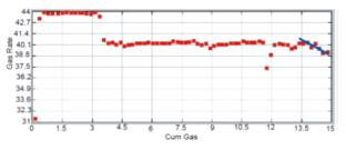
Figure 3. DCA analysis- log (gas rate) versus time for HGF-7
