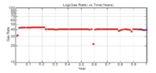
Figure 4. DCA analysis-  $\log$  (gas rate) versus time for HGF-10
