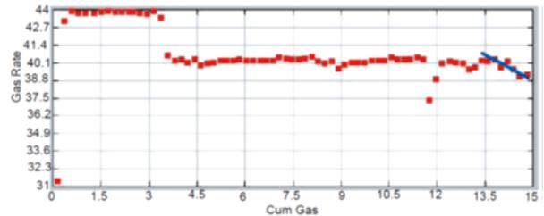
Figure 4. DCA analysis- gas rate versus cumulative gas for HGF-7
