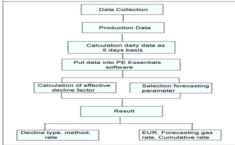
Figure 2. Working procedure of the study
