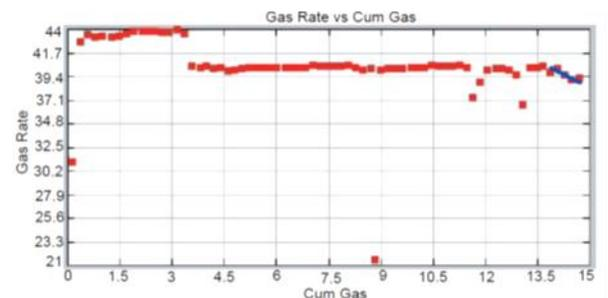
Figure 5. DCA analysis- gas rate versus cumulative gas for HGF-10
