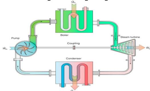
Figure 1. Schematic diagram of Steam turbine system based on Rankine cycle [20].
