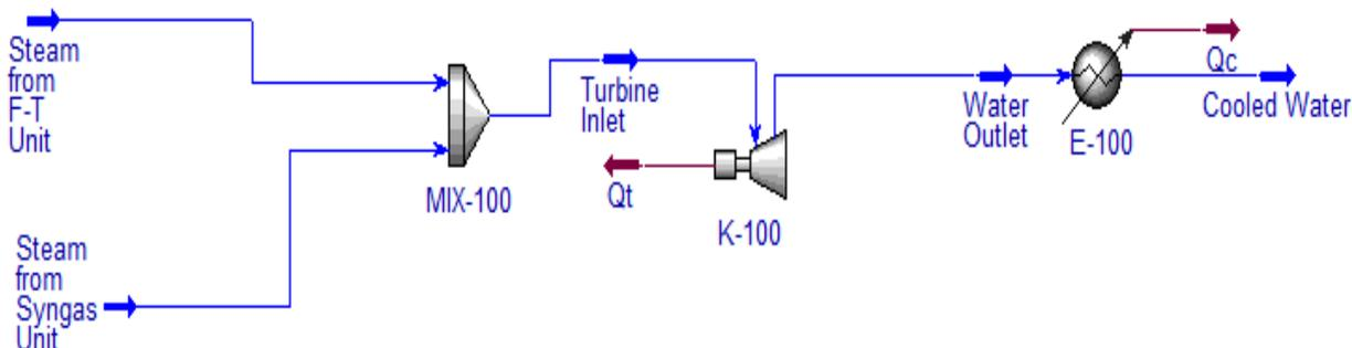
Figure 4. Process flow diagram (PFD)of electricity generation process
