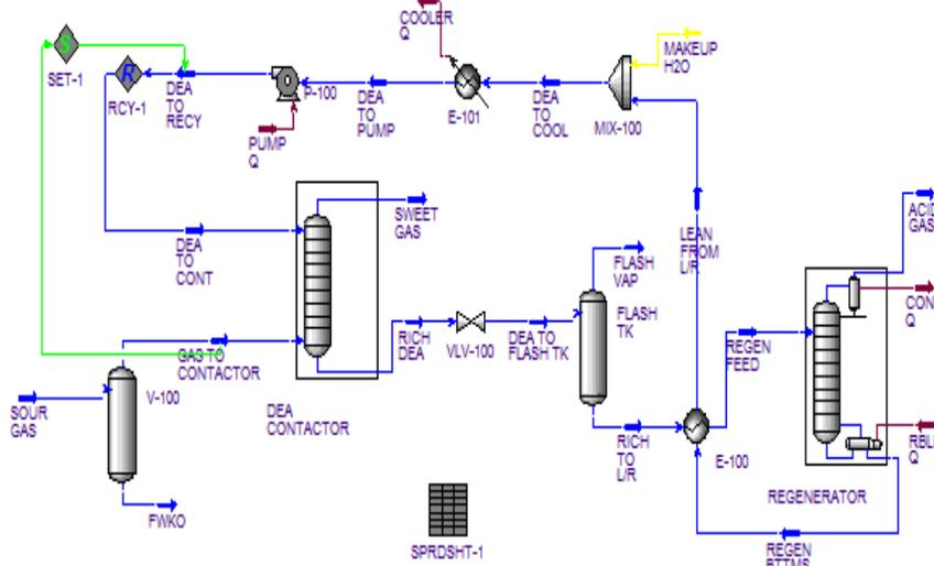
Figure 2. Process flow diagram (PFD) of gas sweetening process using DEA.
