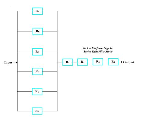
Figure 5 Jacket Structural Reliability Schematic Diagram
