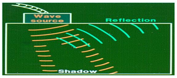
Figure 6 Detection and Reflection of Ultrasonic Beam
