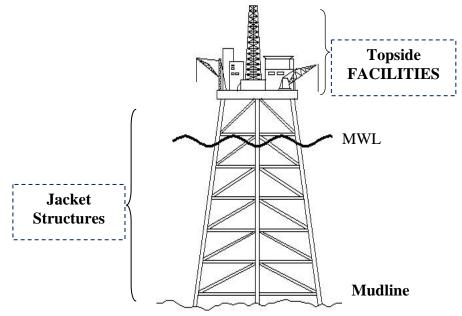
Figure 1 Schematic of Offshore Jacket Platform
