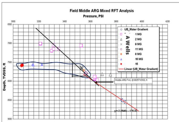
Fig. 4. (a) Middle A/R "G" Free Water Level Determination and
