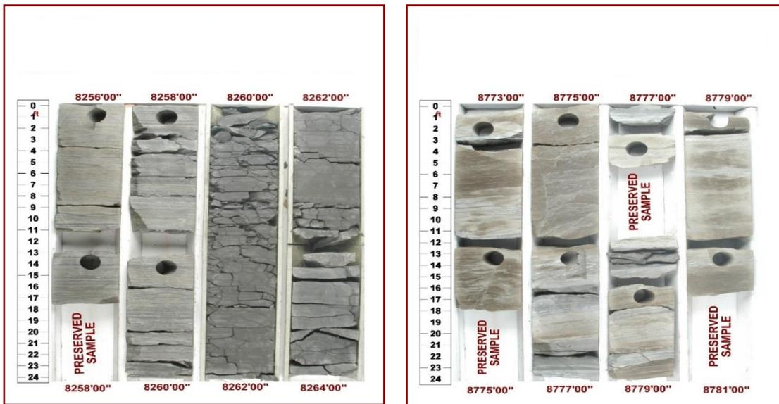
Fig. 2. Middle A/R "G" core and Log sedimentology
