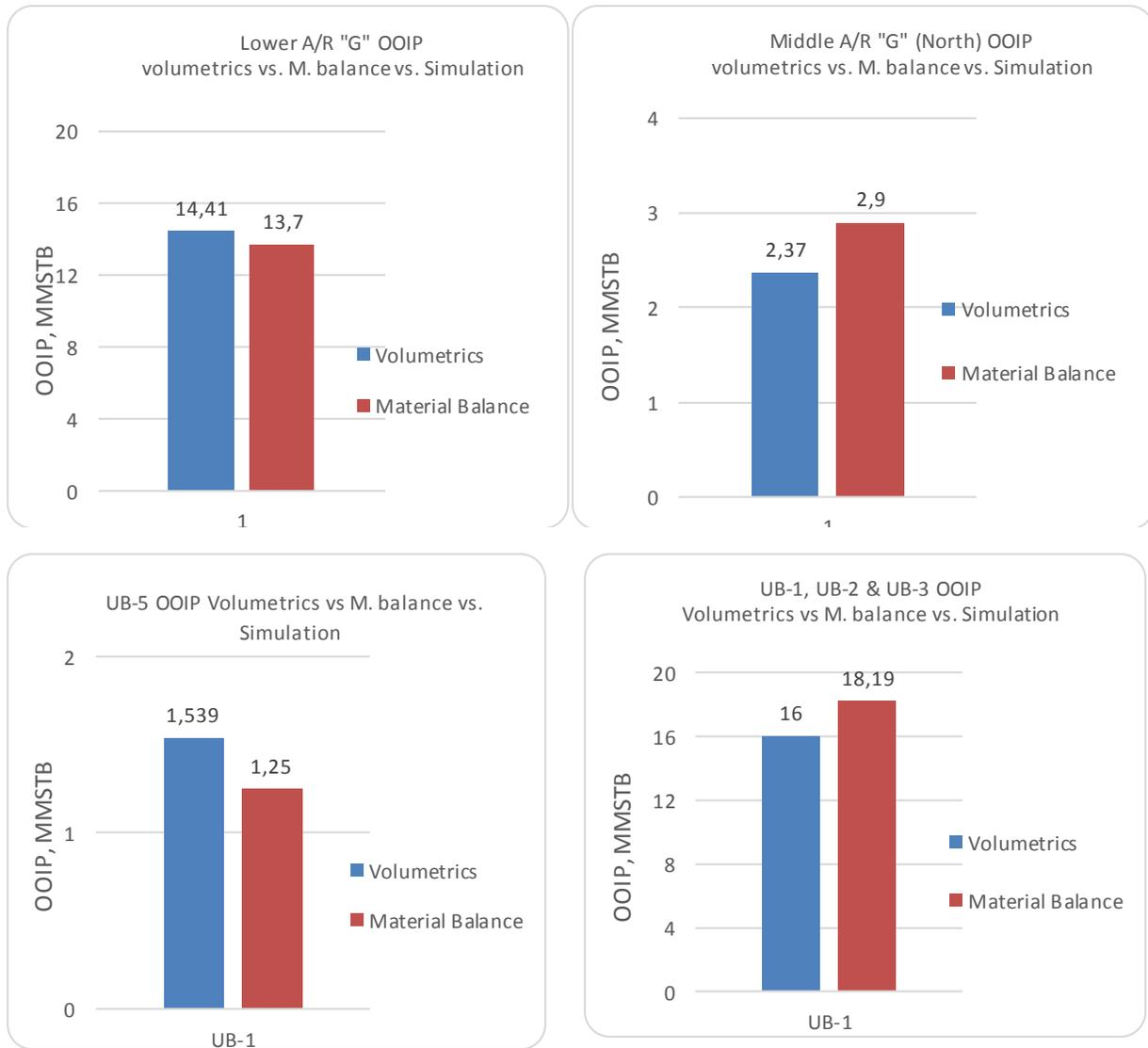
Fig.6. Calculated OOIP using volumetric and MBE method
