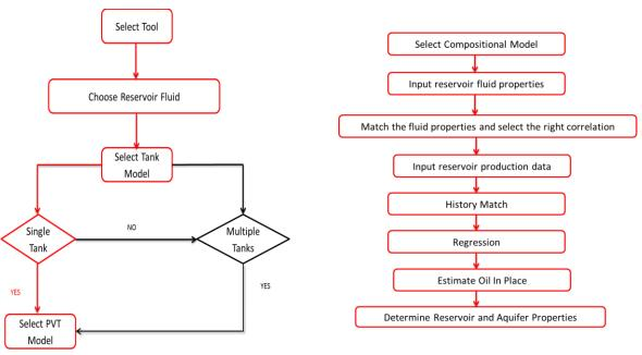
Figure 1a. Material balance workflow in estimating the initial oil in place.
