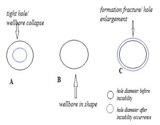
Fig.1. Effect of borehole pressure and horizontal stress ratio on wellbore stability. A. Mud weight lower than the horizontal stress; B. Mud weight equal to the horizontal stress; C. Mud weight higher than the horizontal stress.
