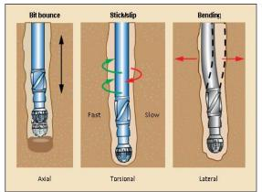
The destructive nature of each type of vibration is different. Lateral vibrations are the most destructive type of vibration and can create large shocks as the BHA impacts the wellbore wall <sup>[30]</sup>. This impact can create cracks in the formation and in some cases, lead to significant hole enlargements. Optimizing bottom hole assembly (BHA) design with respect to the hole geometry, inclination, and formations to be drilled is an important step in controlling drill string vibrations.
