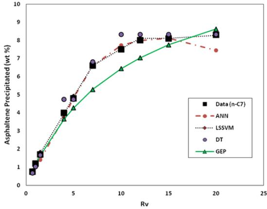
Fig. 6. Trend plot of asphaltene precipitation changes versus dilution ratio at temperature of 30°C for n-C7
