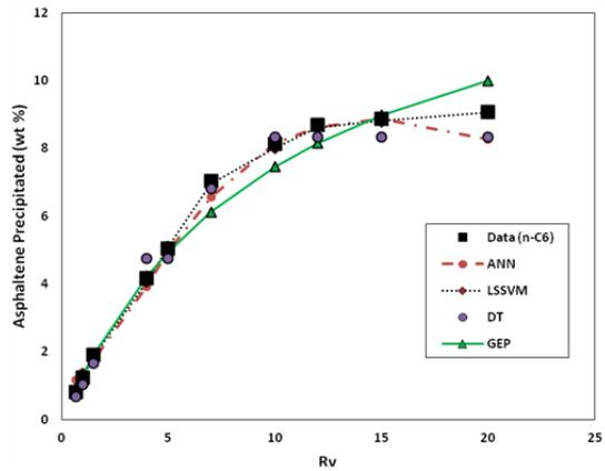
Fig. 5. Trend plot of asphaltene precipitation changes versus dilution ratio at temperature of 30°C for n-C6
