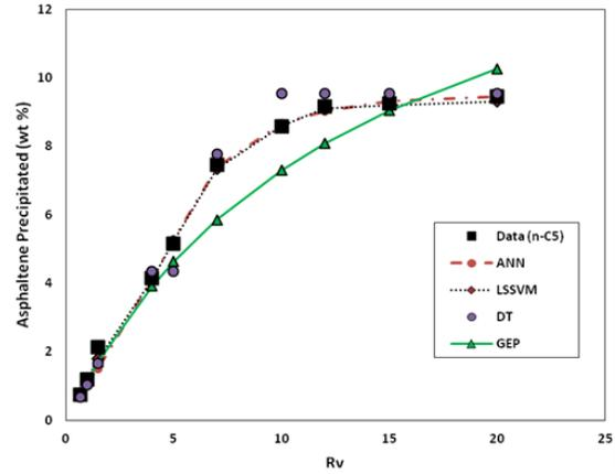
Fig. 7. Trend plot of asphaltene precipitation changes versus dilution ratio at temperature of 50°C for n-C5
