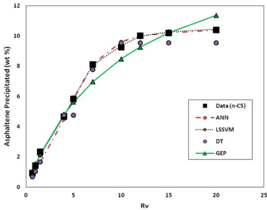
Fig. 4. Trend plot of asphaltene precipitation changes versus dilution ratio at temperature of 30°C for n-C5
