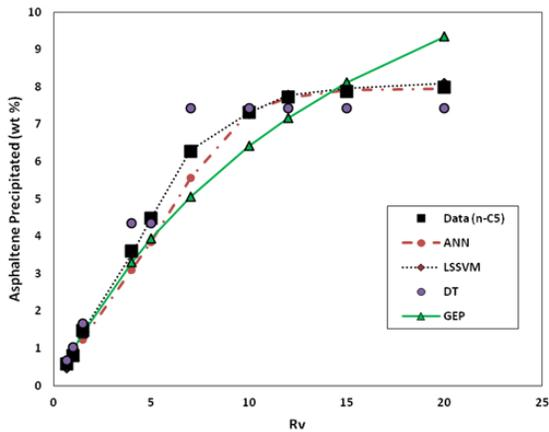
Fig. 10. Trend plot of asphaltene precipitation changes versus dilution ratio at temperature of 70°C for n-C5
