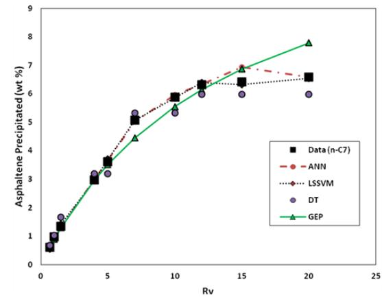
Fig. 9. Trend plot of asphaltene precipitation changes versus dilution ratio at temperature of 50°C for n-C7
