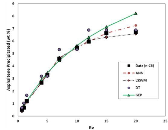
Fig. 11. Trend plot of asphaltene precipitation changes versus dilution ratio at temperature of 70°C for n-C6
