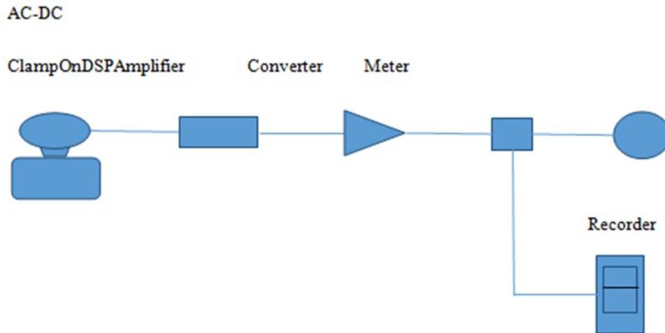
Figure 3. Block diagram showing signal analyzing process of clampOn sand detector.
