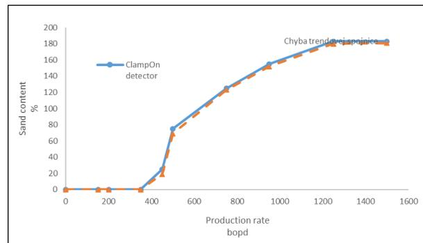
Figure 7. Plot to show results from clampOn sand detector and sampling method for well XD.
