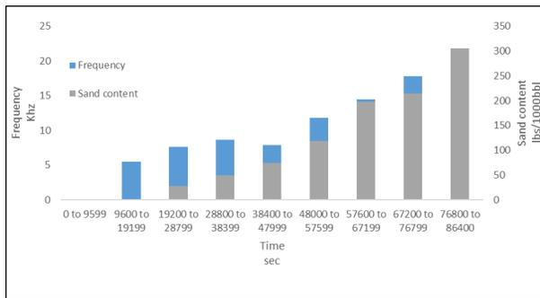
Figure 14. Frequencies to show the corresponding sand detected for well XI.
