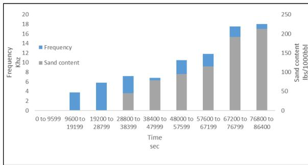
Figure 12. Frequencies to show the corresponding sand detected for well XS.
