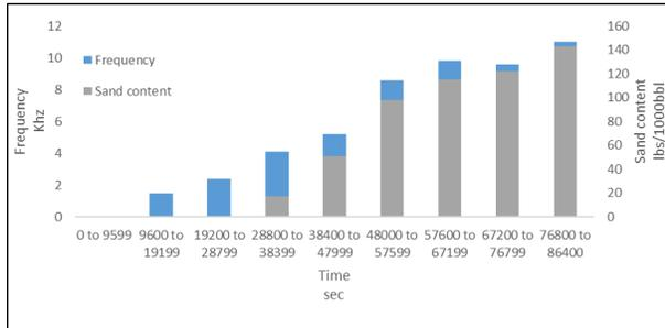
Figure 4. Frequencies to show the corresponding sand detected for well XH.
