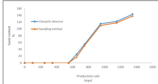
Figure 5. Plot to show results from clampOn sand detector and sampling method for well XH.
