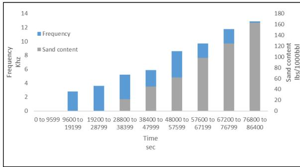
Figure 8. Frequencies to show the corresponding sand detected for well XA.
