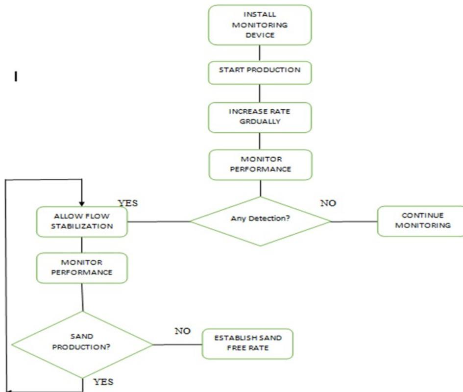
Figure 2. Flow chart for monitoring sand production.
