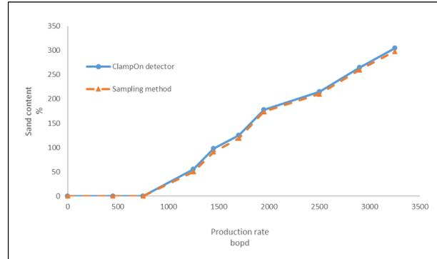
Figure 15. Plot to show results from clampOn sand detector and sampling method for well XI.
