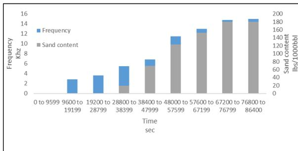
Figure 6. Frequencies to show the corresponding sand detected for well XD.
