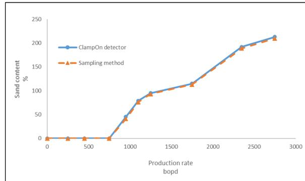
Figure 13. Plot to show results from clampOn sand detector and sampling method for well XS.
