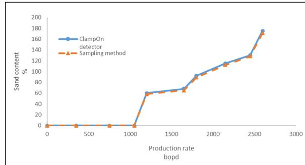
Figure 11. Plot to show results from clampOn sand detector and sampling method for well XX.
