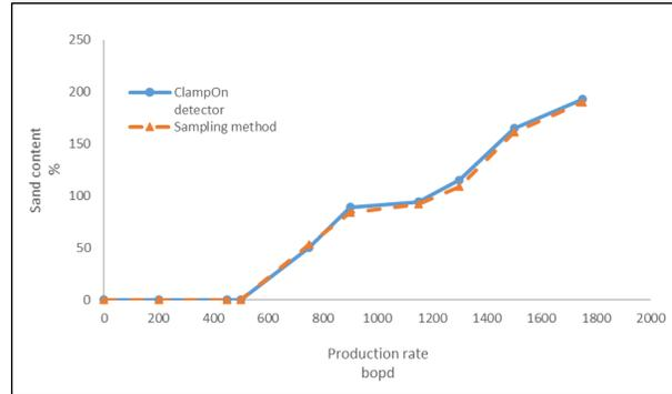
Figure 9. Plot to show results from clampOn sand detector and sampling method for well XA.
