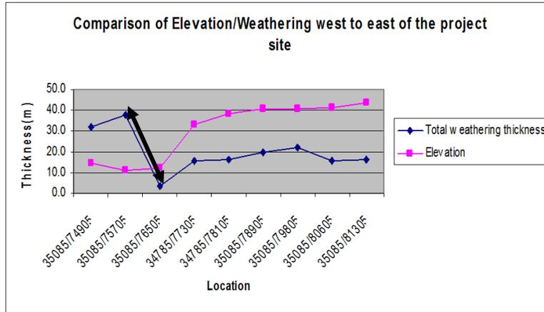
Fig. 11. Comparison of elevation/weathering thickness, west to east of the project area (The black the arrow shows the position of the Sombreiro River)
