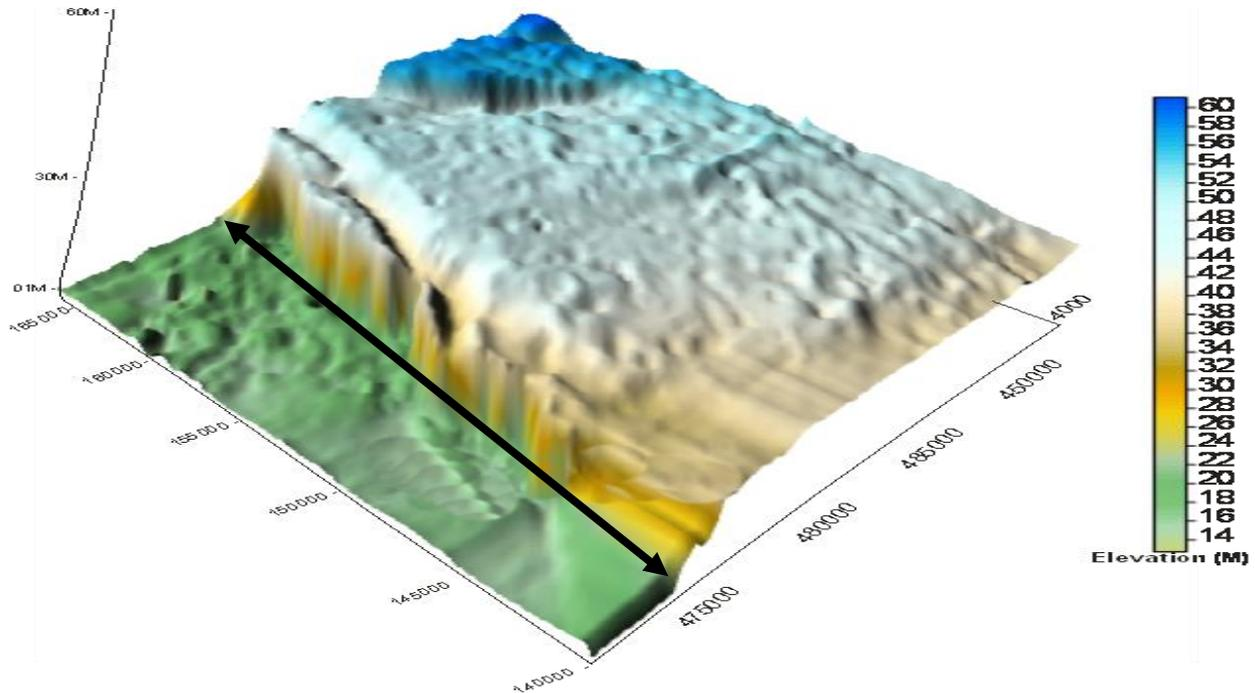
Fig.2. Surface elevation plot of the survey area showing an escarpment (The thick black line indicates where the basin of the Sombreiro River started)
