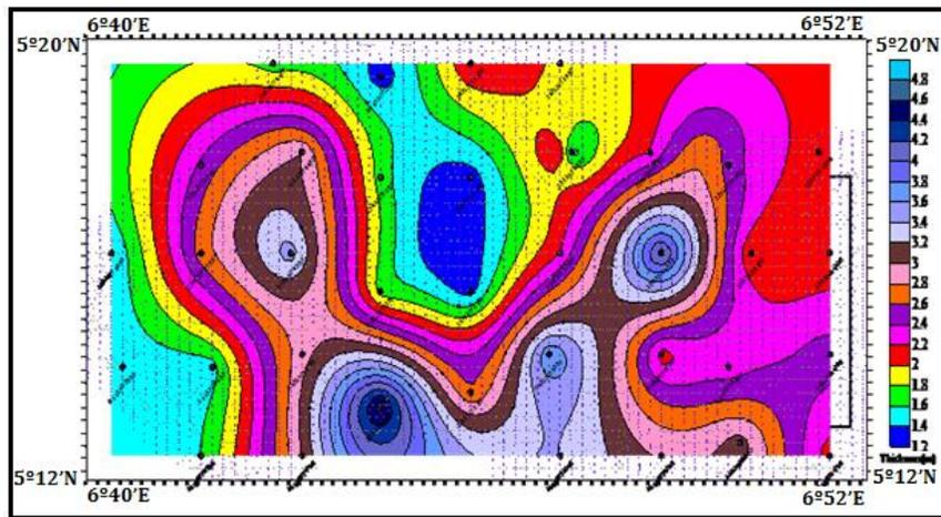
Fig. 9. Weathering layer thickness contour map of the study area
