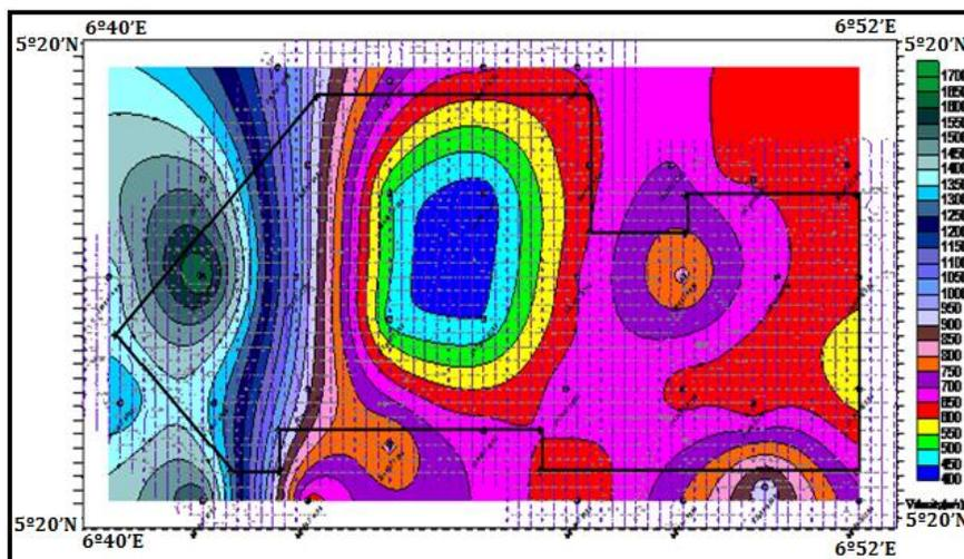
Fig.7. Sub-weathering layer velocity field of the study area
