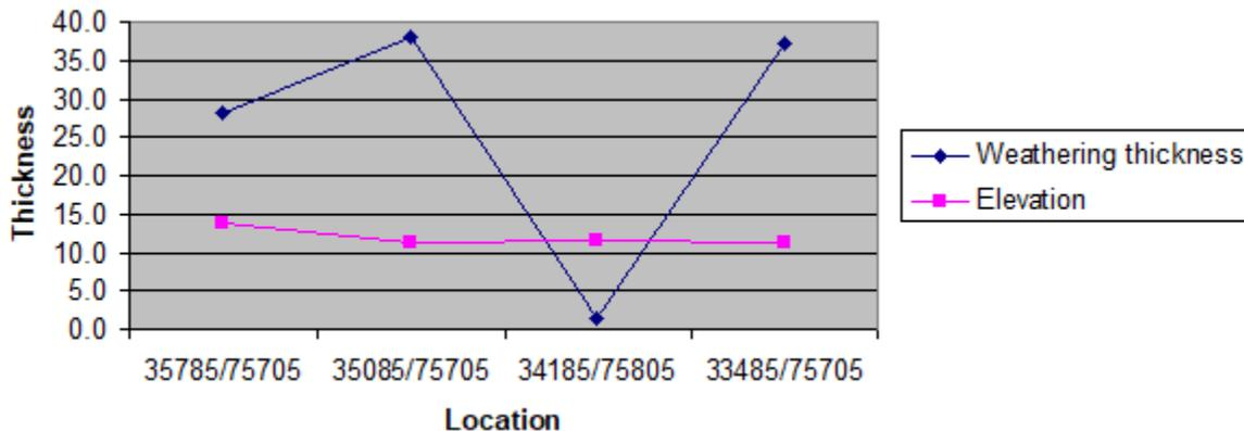
Fig.13. Comparison of elevation and weathering thickness from north to south (west of Sombreiro River)
