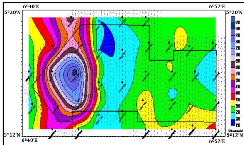
Fig.6. Weathering layer velocity field contour map of the study area
