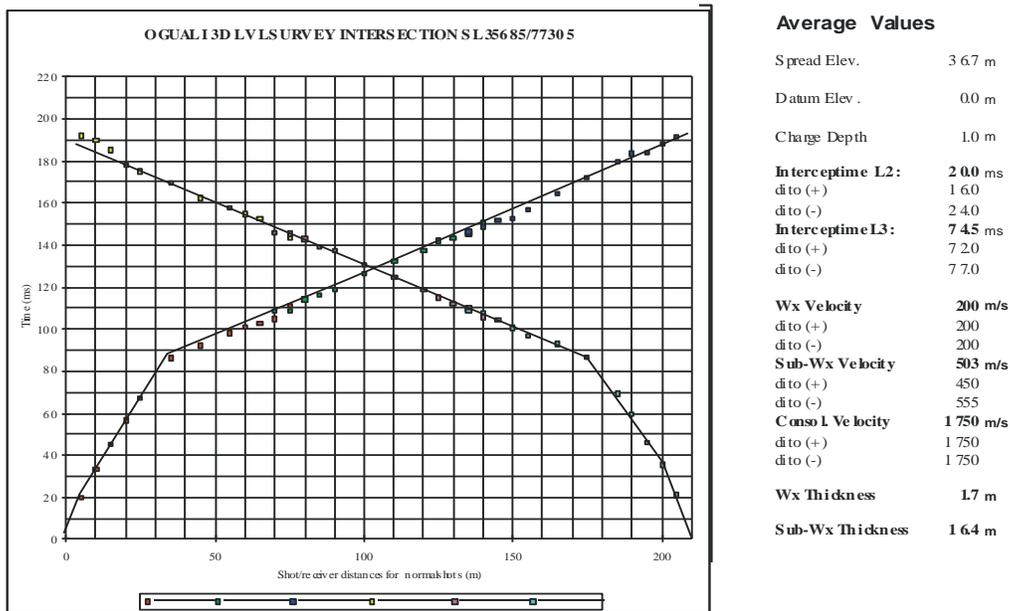
Fig. 4. Typical Time-Distance Plot for LVL survey recorded during the study
