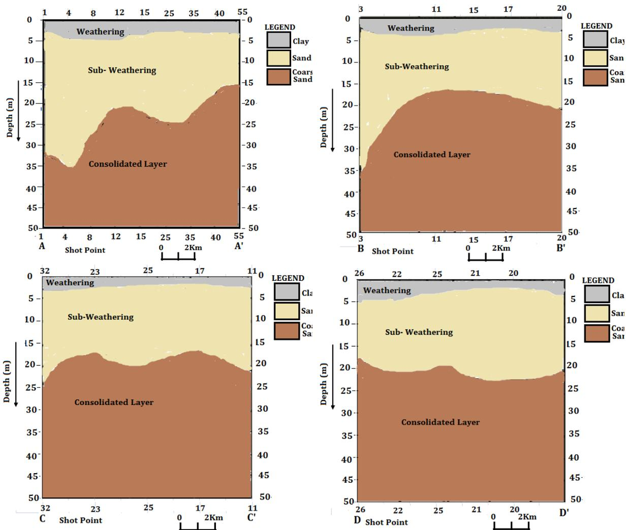
Fig.14. Interpretative cross-sections A- A<sup>1</sup>, B- B<sup>1</sup>, C-C<sup>1</sup> & D-D<sup>1</sup> showing the depth to the weathered layer across the study area
