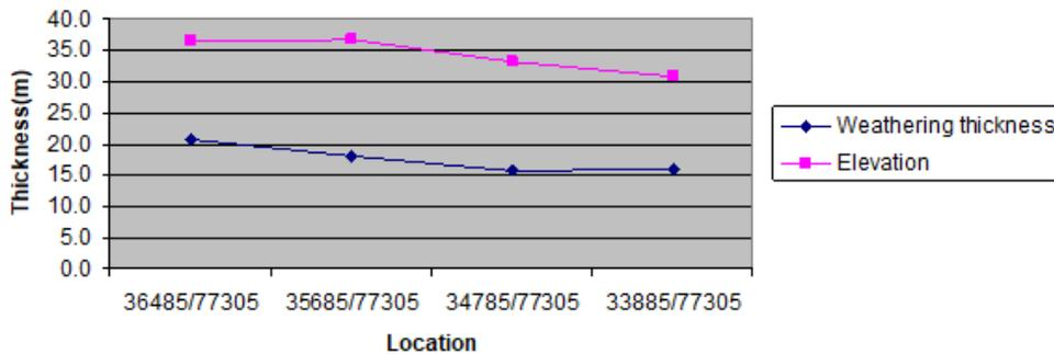
Fig.12. Comparison of elevation and weathering thickness from north to south (east of Sombreiro River)
