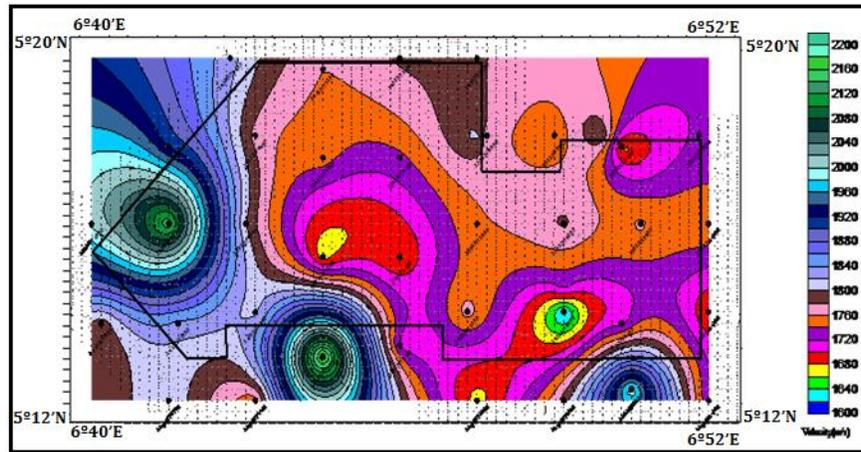
Fig.8. Consolidated layer velocity field of the study area
