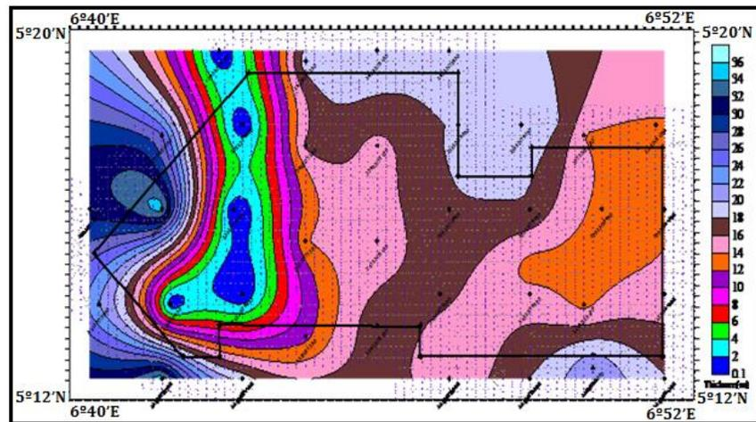
Fig. 10. Sub-weathering layer thickness contour map of the study area
