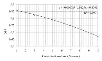
Fig. 2. Dependence of the activity of the dispersion and stabilization oil properties on the concentration of soot particles
