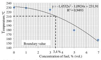
Fig. 3. Dependence of the flash point of the tested oil on the concentration of diesel fuel in it
