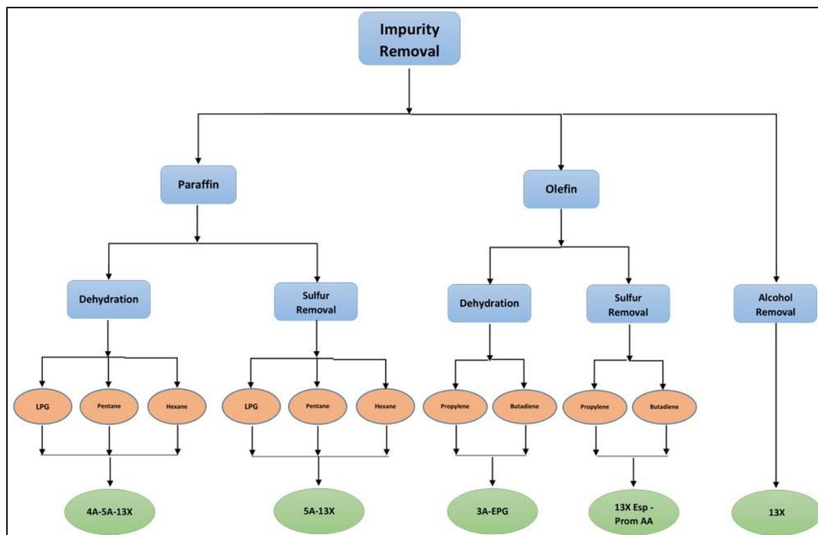
Figure 7. The adsorbent selection diagram (part 4)
