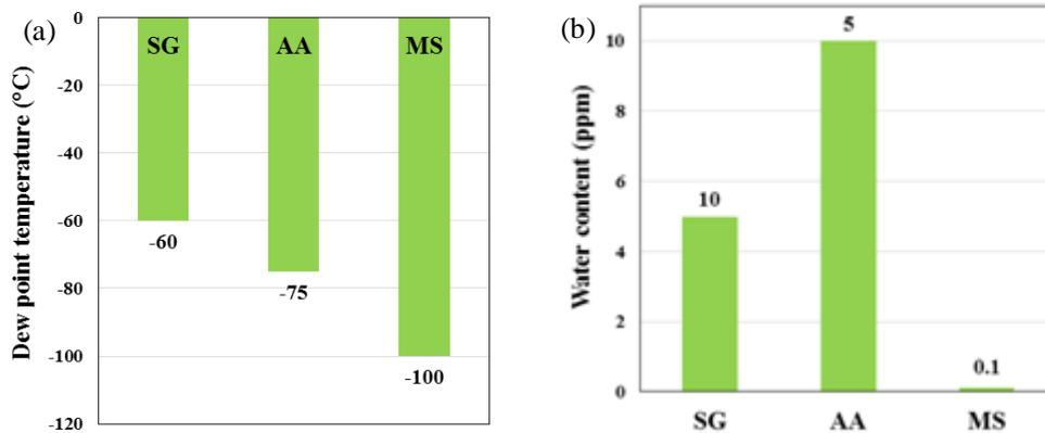
Figure 3. The abilities of SG, AA and MS adsorbents to decrease a) dew point temperature and b) water content of natural gas stream [19]
