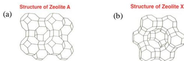
Figure 1. The structure of zeolite A and X type
