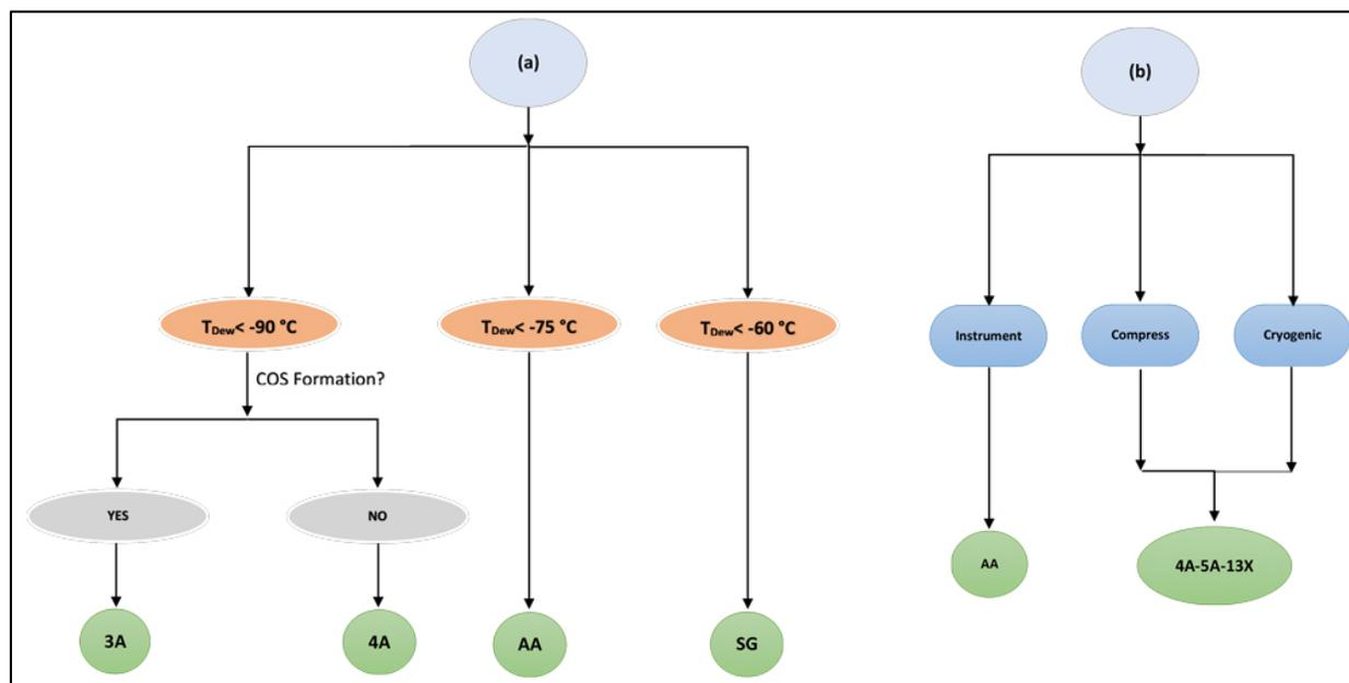
Figure 6. The adsorbent selection diagram (part 3)
