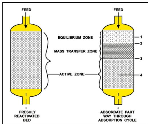
Figure 2. Three zones of an adsorption vessel during adsorption step
