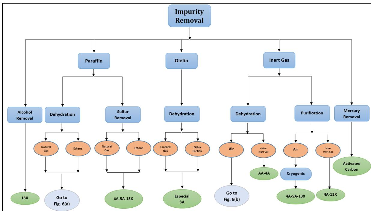
Figure 5. The adsorbent selection diagram (part 2)
