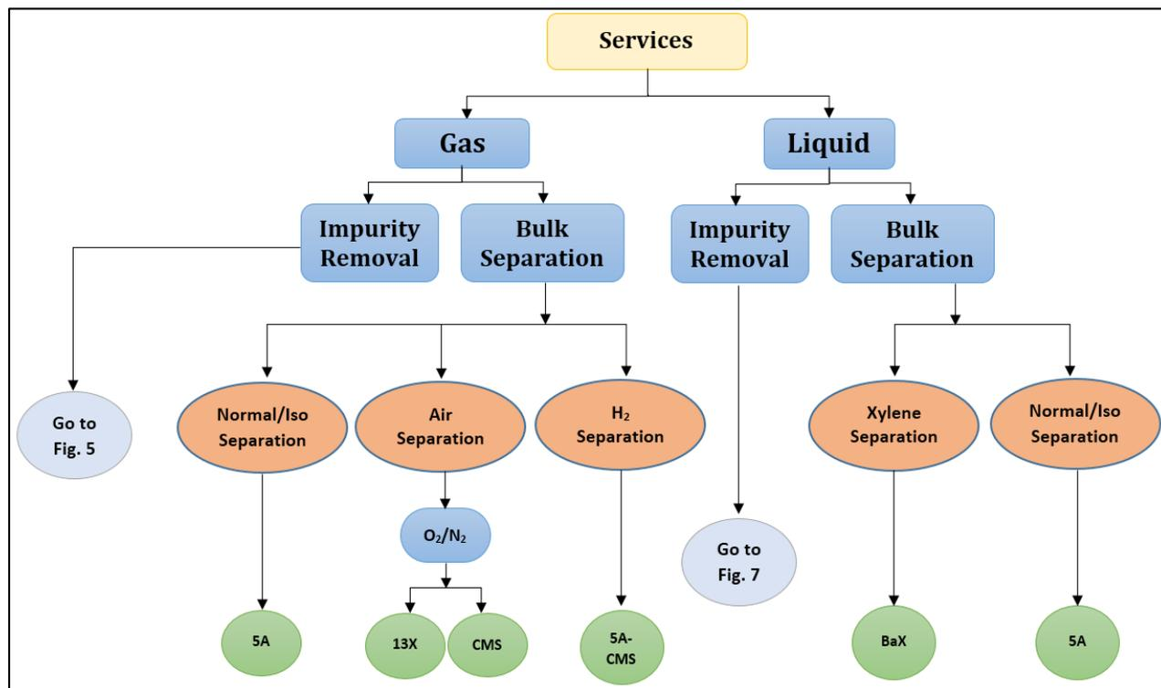
Figure 4. The adsorbent selection diagram (part 1)
