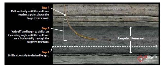
Figure 4. Horizontal drilling [8]
