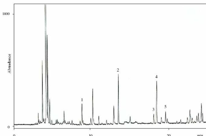
Figure 1. Chromatogram of exposed urine sample. Peaks: 1: benzene (1.07 µg/l), 2: toluene (2.24 µg/l), 3: ethylbenzene (0.49 µg/l), 4: m+p-xylene (1.68 µg/l), 5: o-xylene (0.61µg/l).
