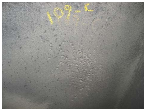
Fig. 2 Pitting Corrosion in L/R amine heat exchanger shell
