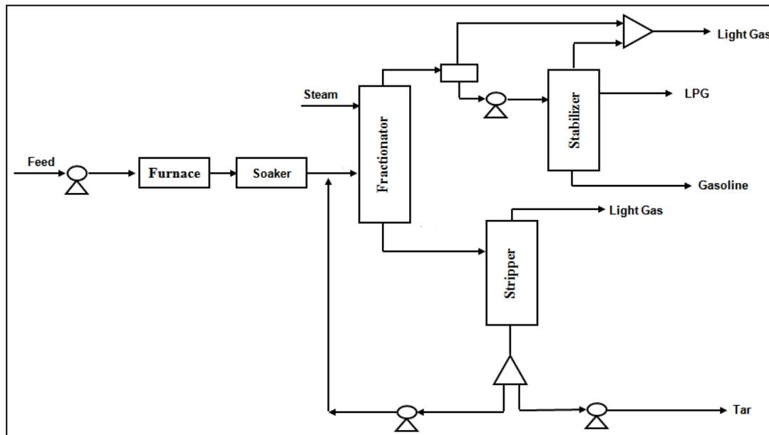
Figure 1 Block flow diagram of visbreaking process
