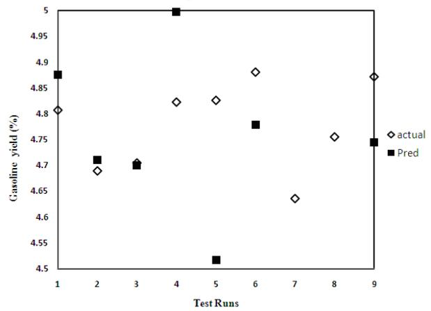
Fig. 6 Comparison between the measured yields and the predicted yield of gasoline.
