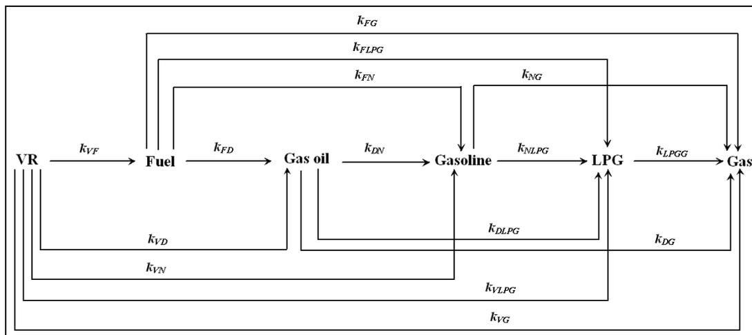
Figure 2 The complete six-lump kinetic model
