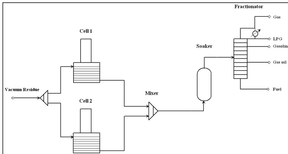
Figure 3 The scheme of the process flow diagram of visbreaking simulator
