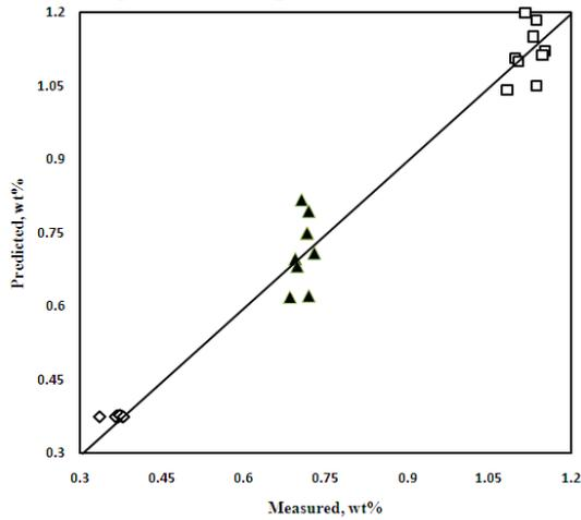
Fig. 5 Comparison between the measured yields and the predicted yields of gas, LPG and gas oil.
