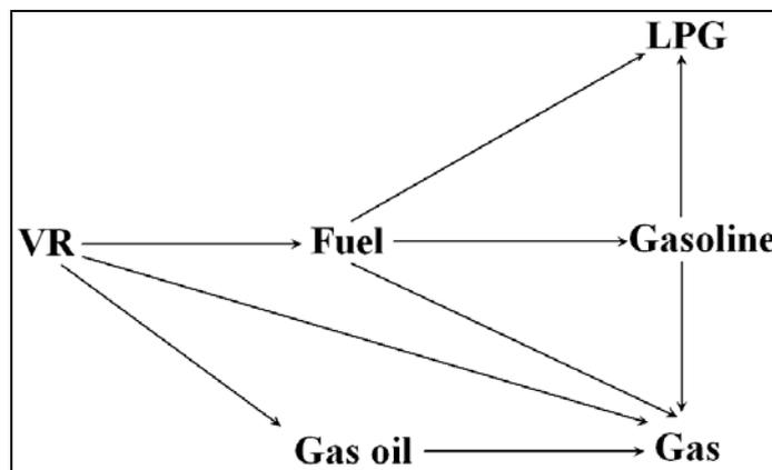
Figure 4 The complete six-lump kinetic model
