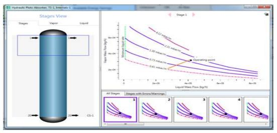
Figure 11. Hydraulics of packed column
