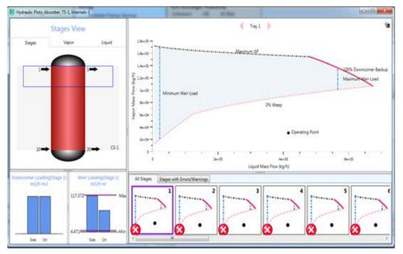
Figure 9. Hydraulic profile of absorber fitted with trays
