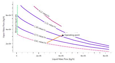
Figure 12. Hydraulic plot for packing column
