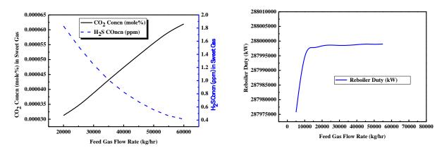
Figure 5. Effect of feed gas flow rate on acid gas concentration in sweet gas
