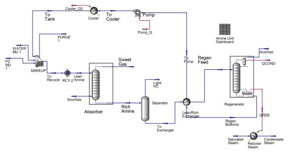
Figure 1. Aspen HYSYS acid gas cleaning flow sheet
