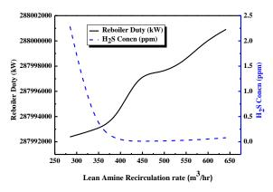
Figure 7. Effect of amine recirculation rate on reboiler duty
