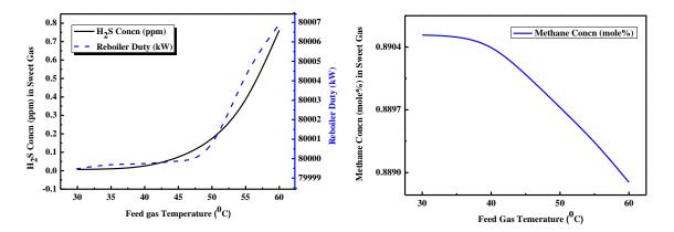
Figure 3. Effect of feed gas temperature on H<sub>2</sub>S concentration in sweet gas
