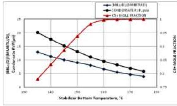
Figure 14. Effect of stabilizer bottom temperature on separation performance
