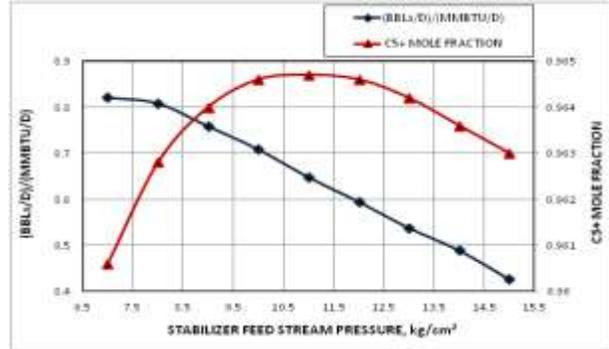
Figure 10. Effect of stabilizer feed stream pressure on separation performance
