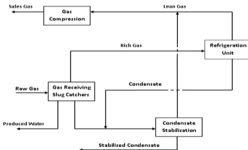
Figure 1. Block diagram for the existing condensate recovery plant
