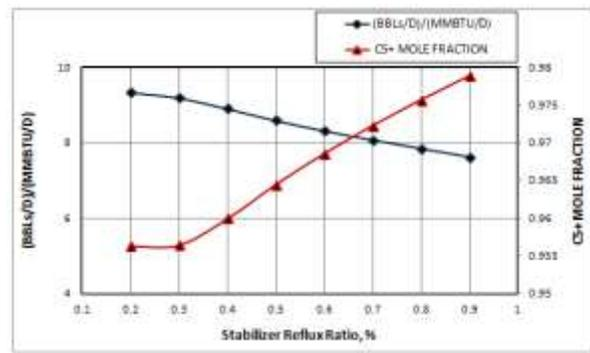
Figure 19. Effect of stabilizer reflux ratio on separation performance
