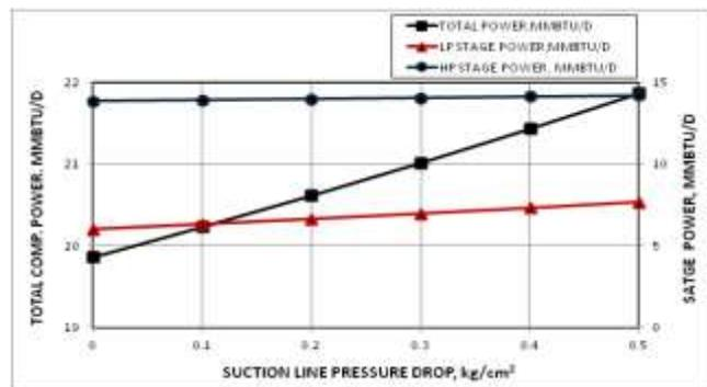
Figure 21. Impact of suction pressure drop on compression power
