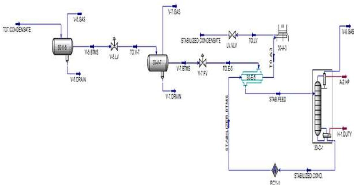
Figure 4. The flow sheet of condensate stabilization section
