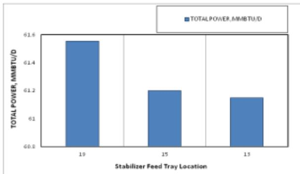
Figure 15. Effect of stabilizer feed tray location on total consumed power
