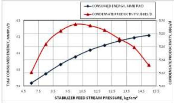
Figures 9. Effect of Stabilizer feed pressure on the objective functions
