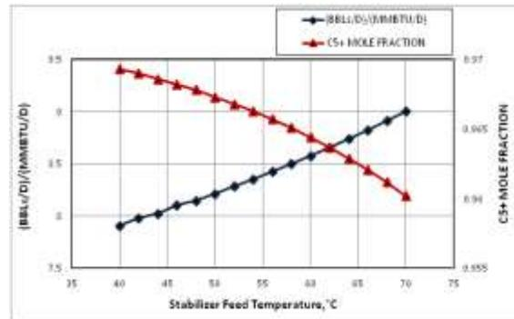
Figure 12. Effect of stabilizer feed temperature on separation performance
