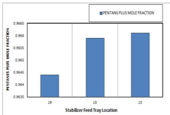
Figure 17. Effect of stabilizer feed tray location on separation performance
