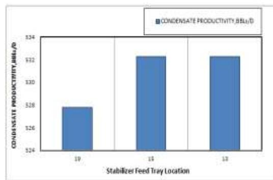
Figure 16. Effect of stabilizer feed tray location on condensate productivity
