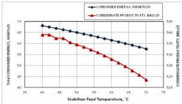
Figure 11. Effect of Stabilizer feed temperature on the objective functions
