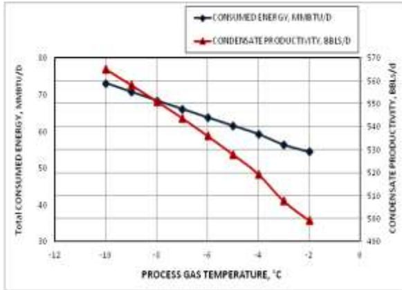
Figures 5. Effect of process gas temperature on process objective functions
