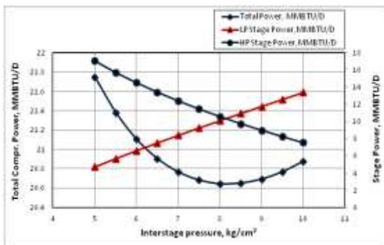
Figure 20. Impact of inter stage pressure on compression power
