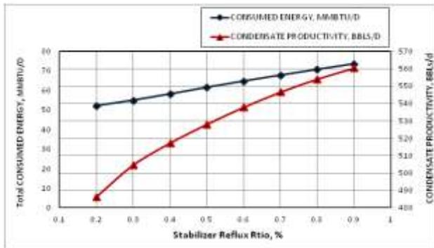
Figure 18. Effect of reflux ratio on the objective functions
