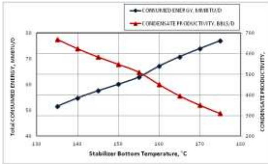
Figure 13. Effect of Stabilizer bottom temperature on the objective functions
