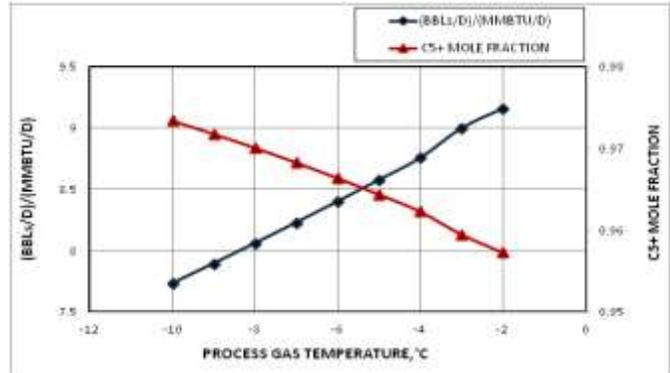
Figure 6. Effect of process gas temperature on separation performance
