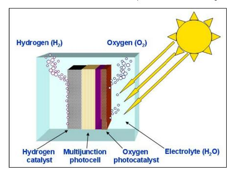
Figure 4: Basic structure of a Photoelectrode
