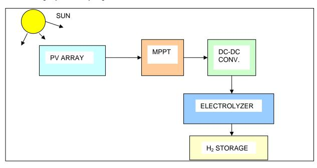
Figure 2 : Schematic of PV – hydrogen production system<sup>[5]</sup>
