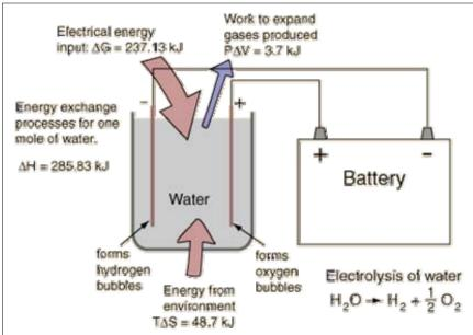
Figure 1: Electrolysis scheme
