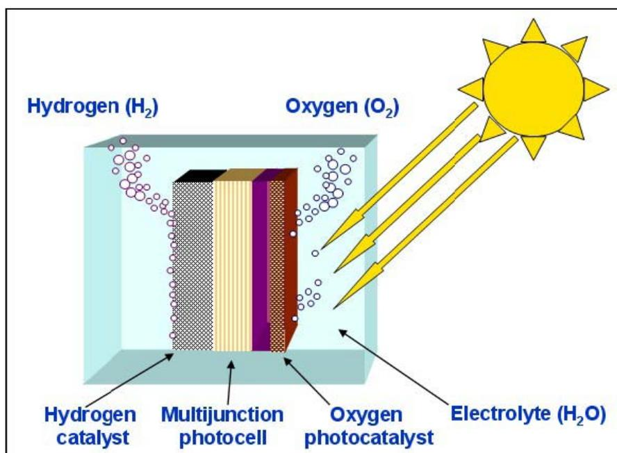
Figure 4: Basic structure of a Photoelectrode
