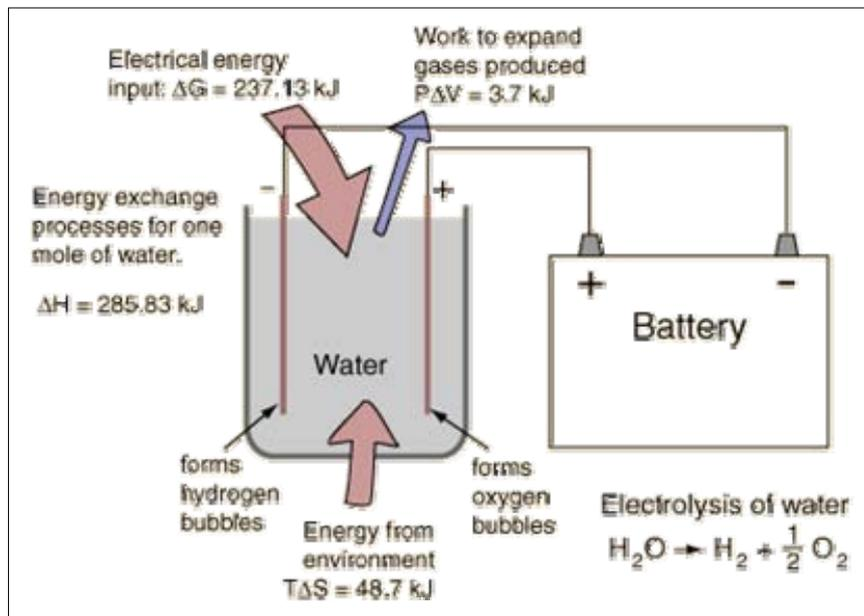
Figure 1: Electrolysis scheme
