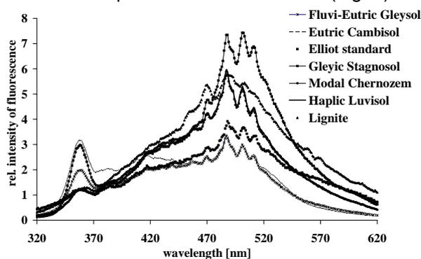
Fig.5 Synchronous fluorescence spectra of HS originated from different sources
