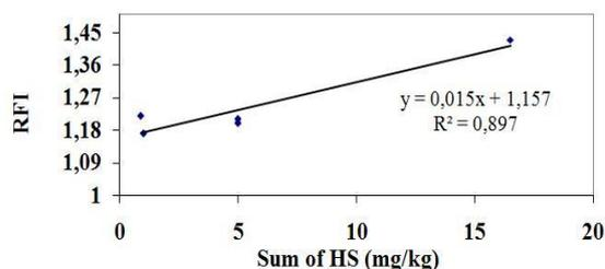
Fig.6 Correlation between RFI indexes (I501/I478) and fractional composition of HS
