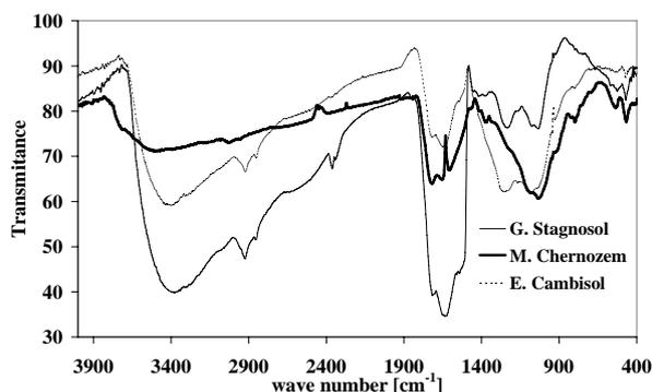
Fig.3 FTIR spectra of HA isolated from Gleyic Stagnosol, Modal Chernozem and Eutric Cambisol
