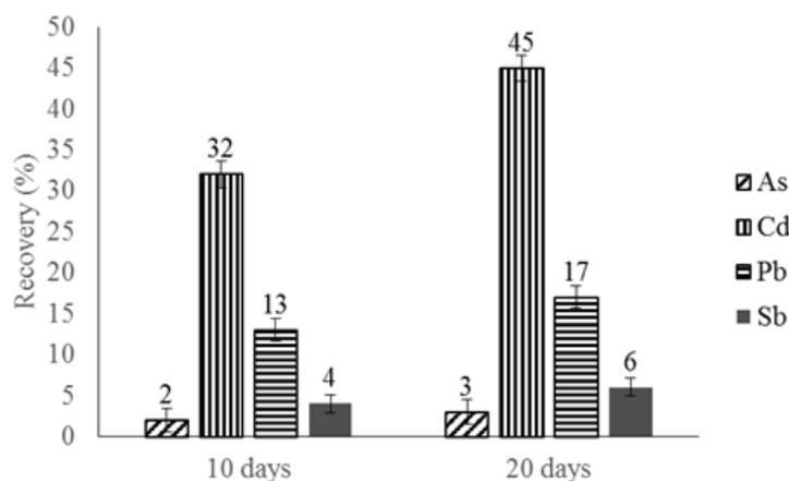
Fig. 3. Recovery of As, Cd, Pb and Sb from printed circuit boards (PC boards) after 10 and 20 days bioleaching by *Acidithiobacillus ferrooxidans*. All values are in mean ( $n = 3$ )  $\pm$  S.D
