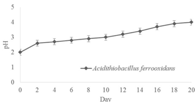
Fig. 1. Variation in pH during PC boards bioleaching by *Acidithiobacillus ferrooxidans*. All values are in mean ( $n = 3$ )  $\pm$  S.D.
