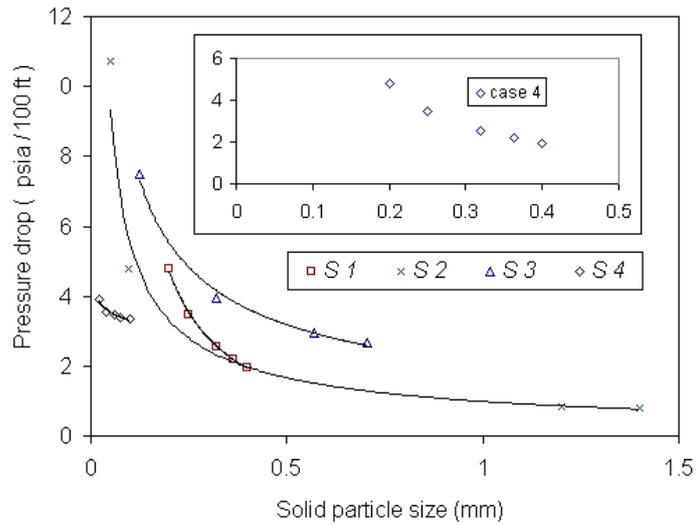
Figure 2. Pressure drop curve versus solid particle size
