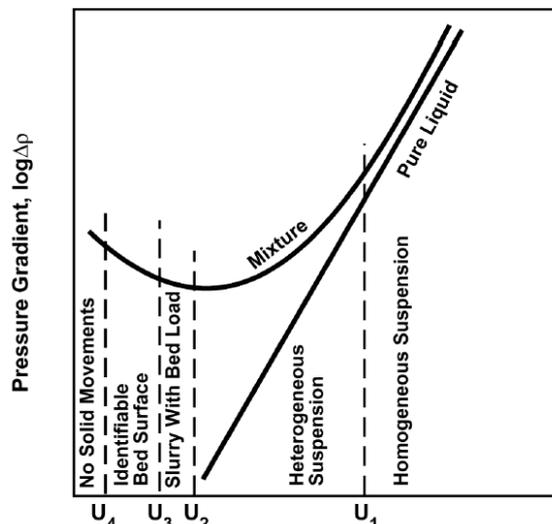
Figure 1. Pressure Drop Variation versus Velocity
