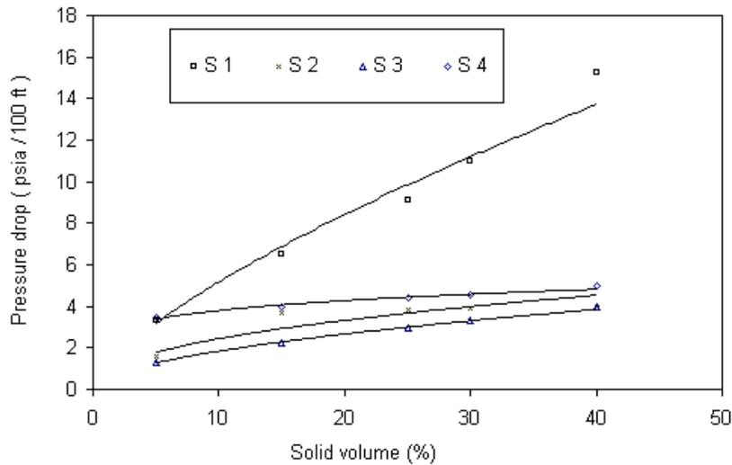
Figure 3. Pressure drop curve versus solid volume
