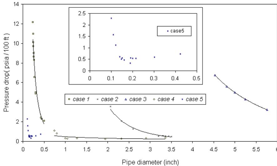
Figure 5. Pressure drop curve versus pipe diameter
