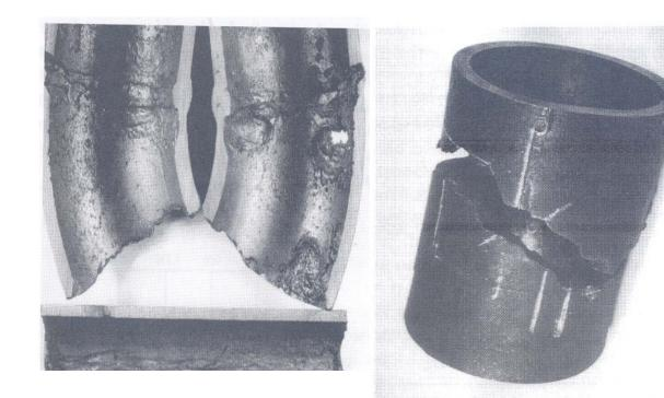
Figure 4-Typicall CO<sub>2</sub> corrosion in pipe
