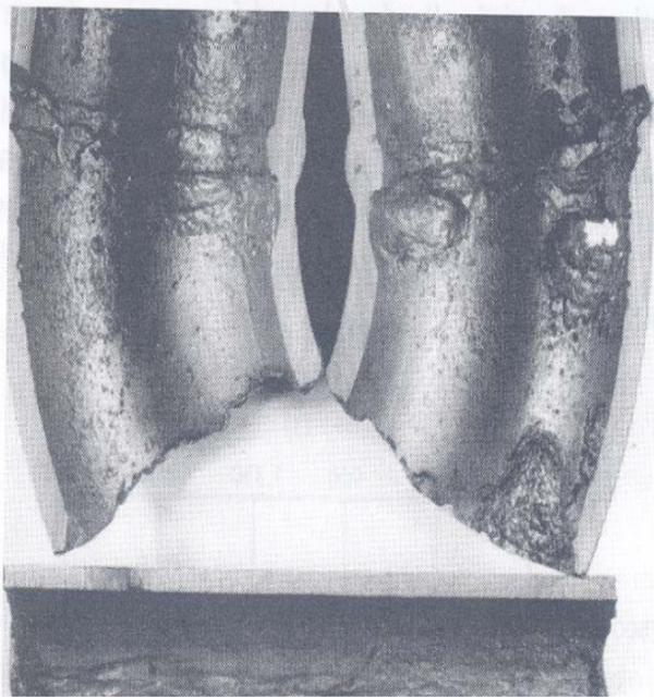
Figure 4-Typical CO<sub>2</sub> corrosion in pipe
