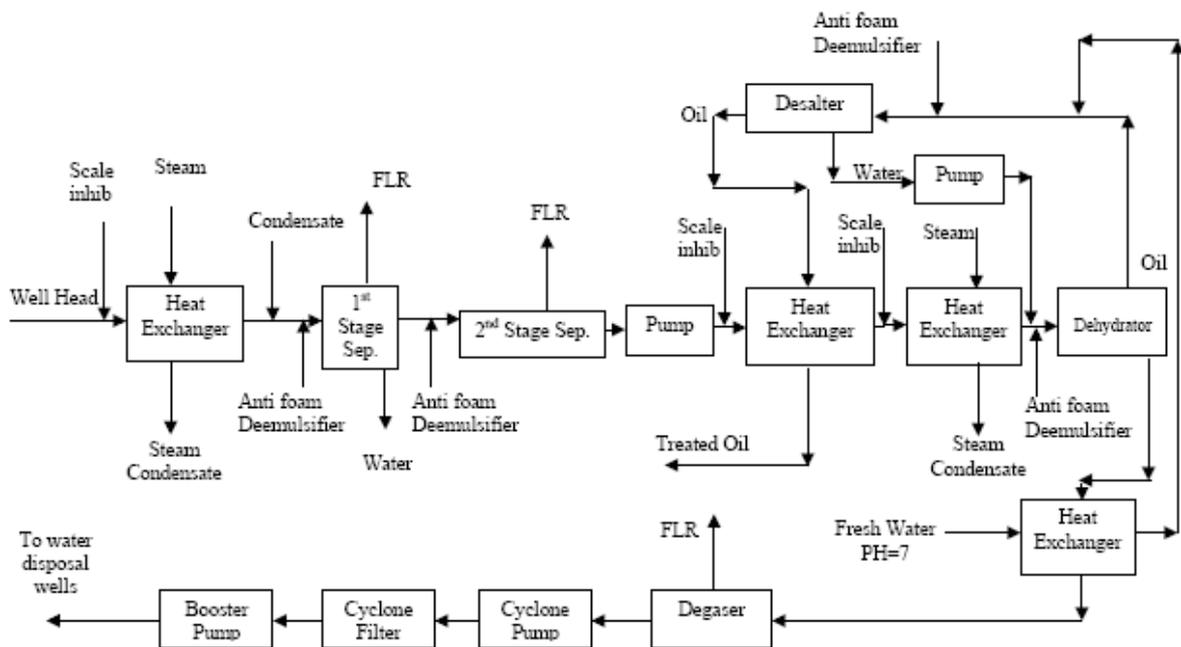
Figure 1- Offshore Oil Production Unit.
