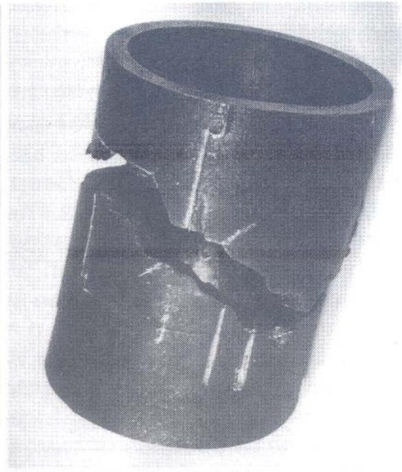
Figure 5-Pipe cracking caused by H<sub>2</sub>S.
