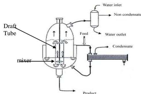
Fig. 1 – Schematic diagram of a DTB crystallizer
