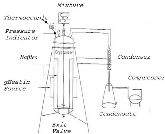
Figure 2: General scheme of crystallizer, which used in the research
