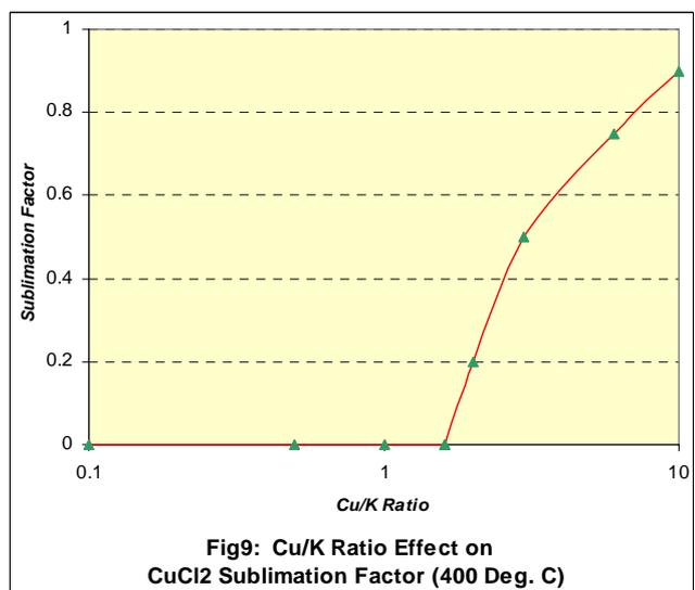
Fig9: Cu/K Ratio Effect on CuCl<sub>2</sub> Sublimation Factor (400 Deg. C)
