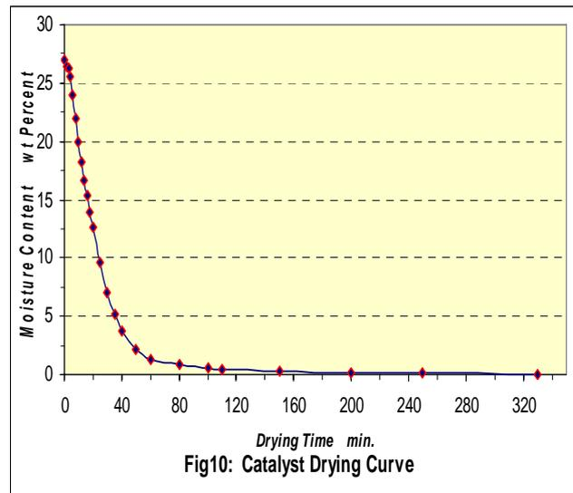
Fig10: Catalyst Drying Curve
