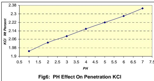
Fig6: PH Effect On Penetration KCl
