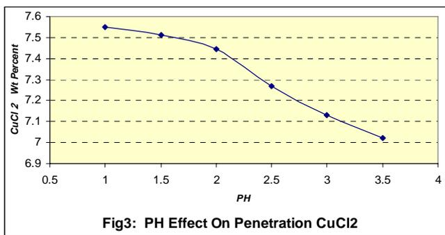
Fig3: PH Effect On Penetration CuCl<sub>2</sub>
